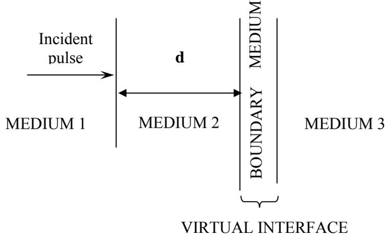
**Figure 2:** Ultrasonic pulse incident upon layered media [1].
