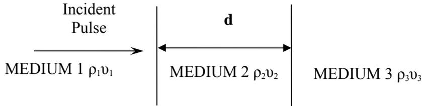
**Fig.1.** Ultrasonic pulse incident upon medium of finite thickness [1].
