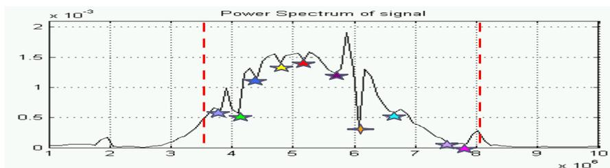
**Figure. 4.A** The experimental graph of power spectrum of the compartment composed of 4 plates of Steel and Aluminum: St-Al-St-Al
