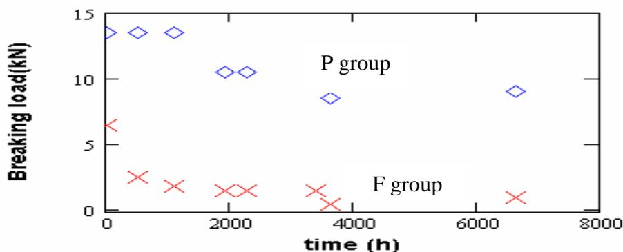
Figure 1: The breaking load of the specimens versus the time of exposure to the hot water
