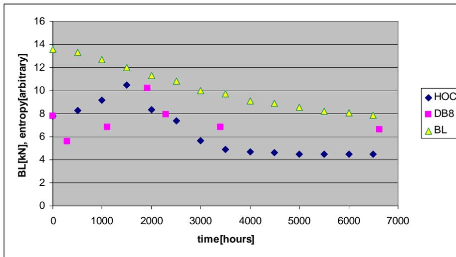
**Figure 6:** The entropy's turning-point pattern obtained from both the DB8-transform and the HOC white-noise test. The breaking-loads of the specimens are plotted as well, as a function of the immersion time.
