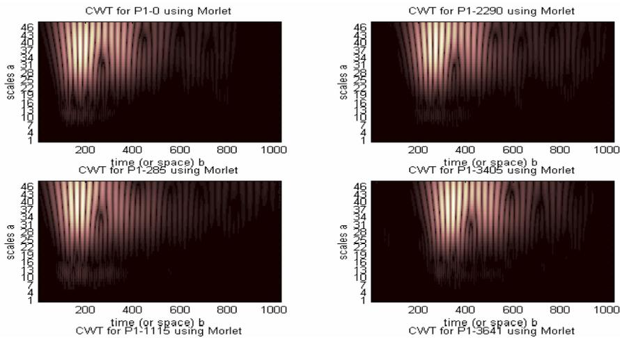
**Figure 3:** CWT of the signals received from one of the P-specimens following different times of exposure to hot water (0, 285, 2290 and 3405 hours) using Morlet Wavelet
