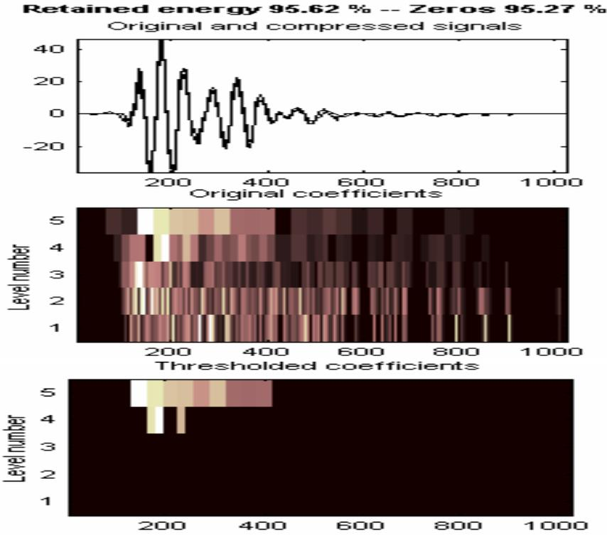
**Figure 4.:** Compressing after DWT of one of the Ultrasonic signals from one of the P specimens
