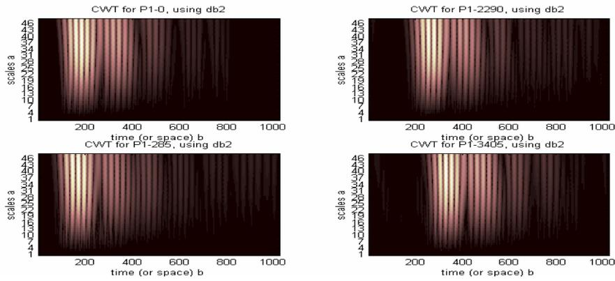
**Figure 2:** CWT of the signals received from one of the P-specimens following different times of exposure to hot water (0, 285, 2290, 3405 hours), using db2 Wavelet
