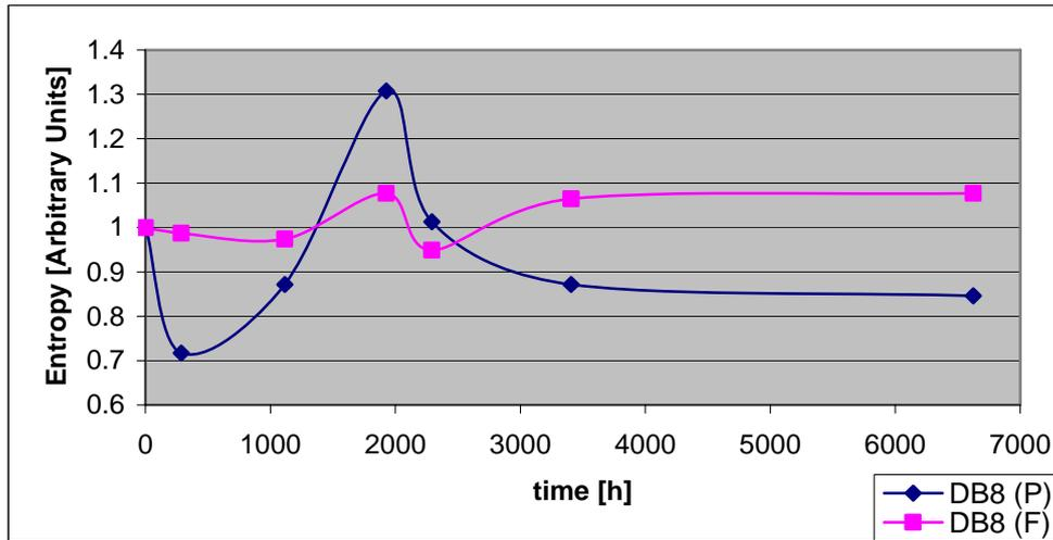
**Figure 5:** The values of average Shannon entropy for the signals from P and F specimens, using DB8 discrete wave transform versus the time of immersion in hot water.
