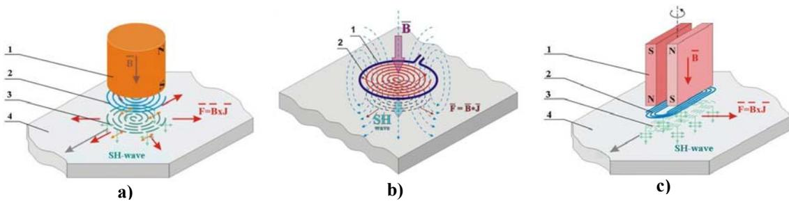
**Fig. 1.** Scheme of shear waves excitation with EMATs with radial polarization – with constant magnet- a) and pulse-magnetic biasing - b), and with linear polarization with constant magnet - c)
