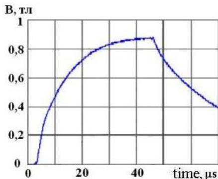
**Fig. 2.** Relation between magnetic field induction n and time in the area close to EMAT surface.
