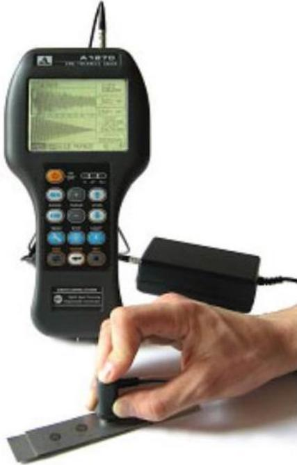
**Fig.9.** Process of weld testing with pulse-magnetic biasing EMAT
