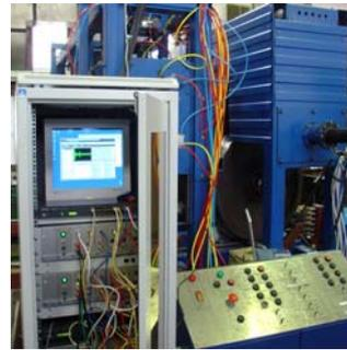
**Fig. 13.** Multi-channel flaw detector A2001 BASIS
