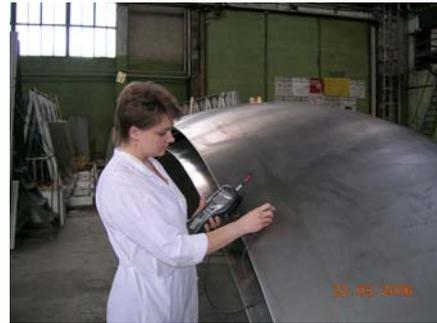
**Fig. 4.** Thickness measurement on big size objects
