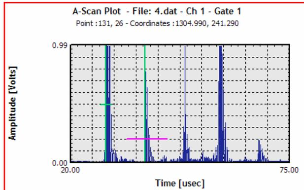
Figure 5: Recording second back wall echo for paint thickness removal.
