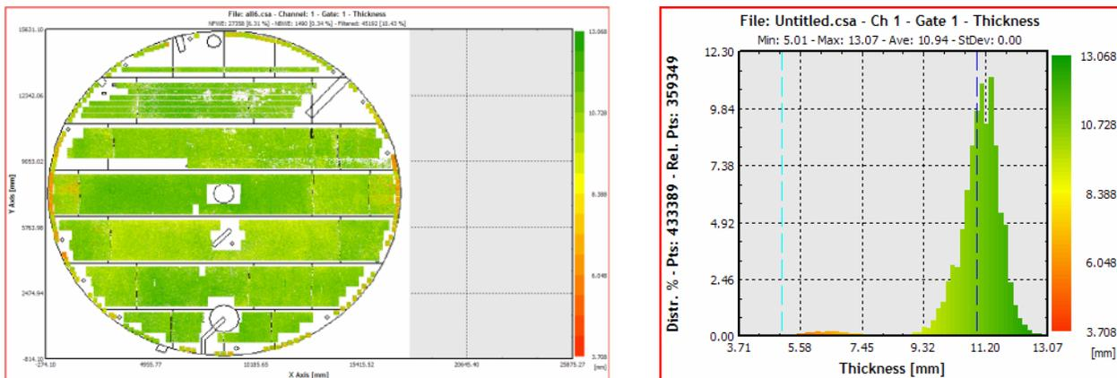
Figure 3. Tank floor composite scan. More than 200 individual scans were used to produce the composite image of more than 438,000 measurements.
