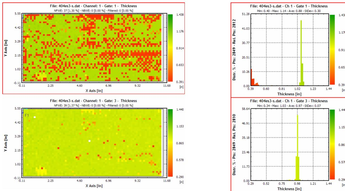
Figure 1. Example of the use of the Reflections strategy. The large number of NRI (red) in the top picture is not there when using the “Reflections” technique for thickness measurement (bottom picture). The respective histogram of thickness distribution is presented next to each C-Scan.
