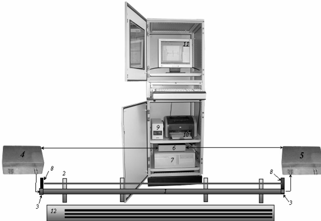
Fig.1. **The scheme of technology realization:** 1 -extended object, 2 - testing rack, 3 - source and receiver electroacoustic sensors, 4,5 - generator and preamplifier units, 6 - control and switching unit, 7 - PC system with ADC, 8 - laser roulette with a reflector, 9 - UPS unit, 10 - printer, 11 - monitor, 12 - rack for rejected objects
