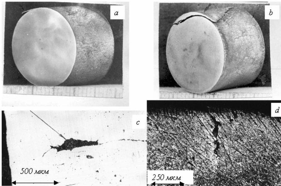
Fig. 3. Microsection metallographic specimens of some defects in the pump rods  $\varnothing 19$  mm: a - rolling defect - fold, b- steelmaking defect - scab, c - slag inclusion, d - hair seams
