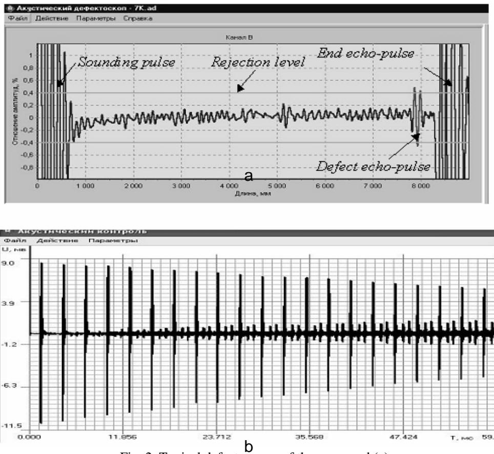
Fig. 2. Typical defectograms of the pump rod (a) and the pump-compressor tube (b) with local defect
