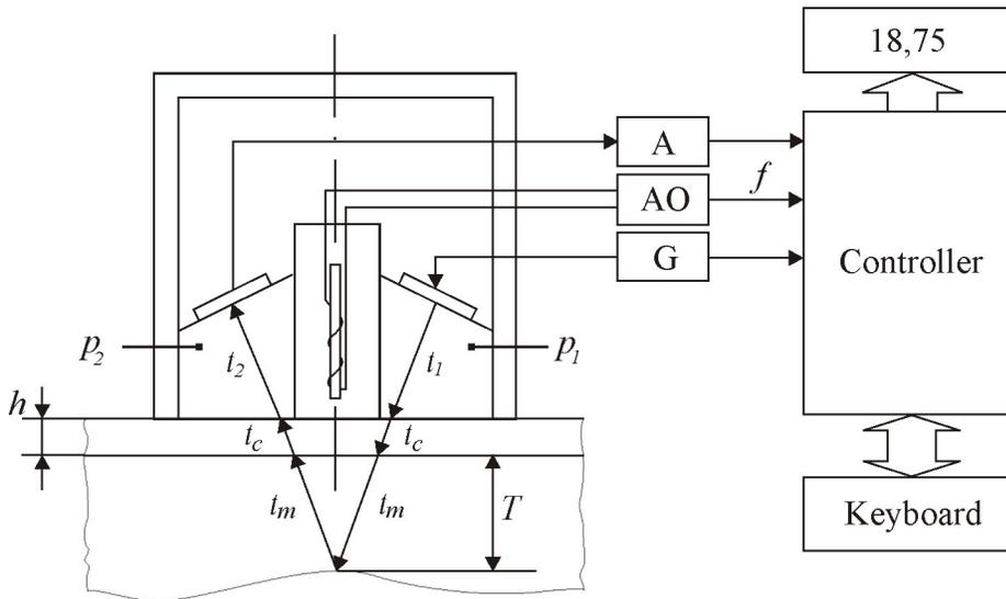
Figure 4. Structure of measuring converter for nonferromagnetic metals.
