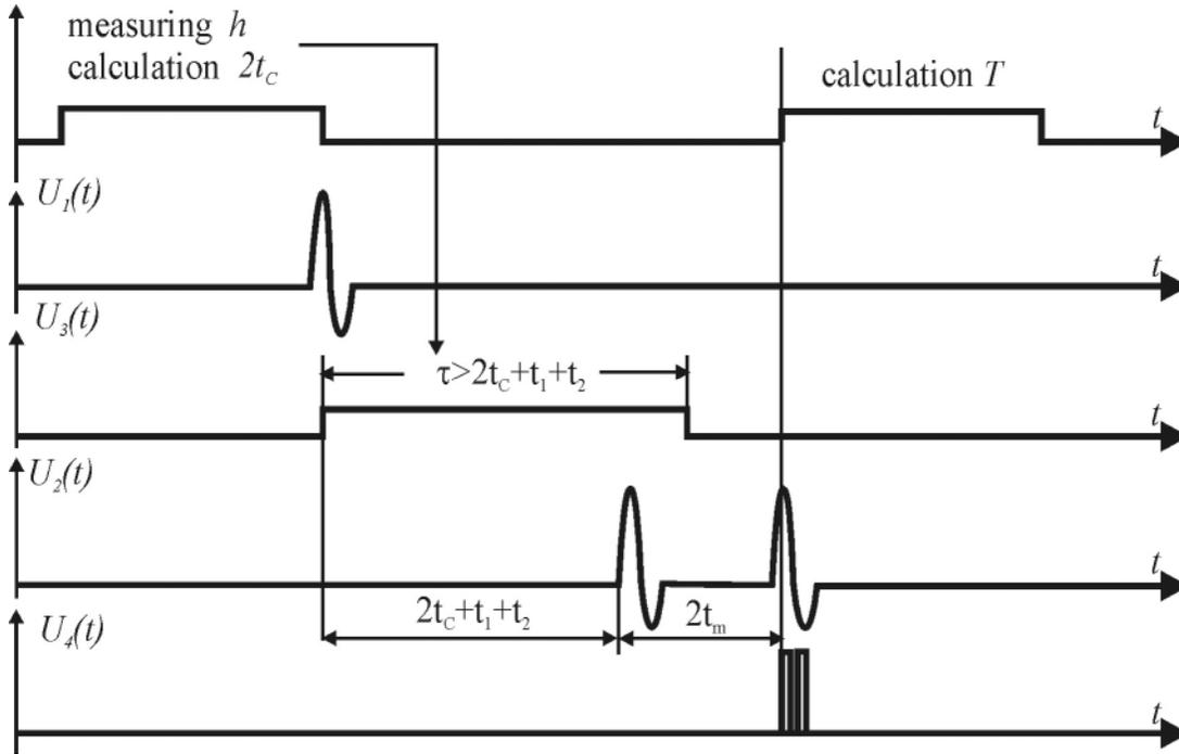
Figure 3 Chart, illustrating operation of combined converter during measuring of residual metal thickness  $T$
