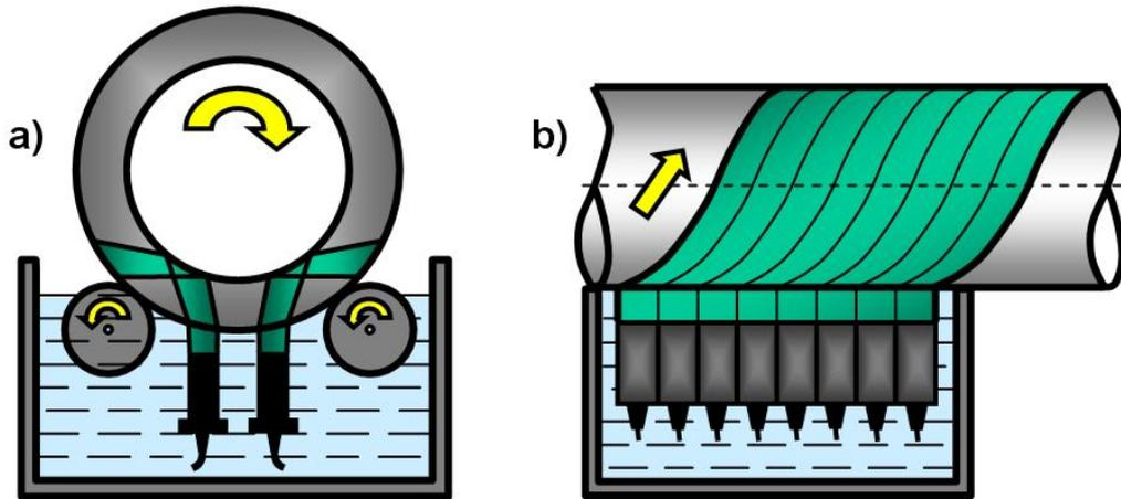
Fig. 2: RPS.R-Echograph rotational tube test in partial immersion
