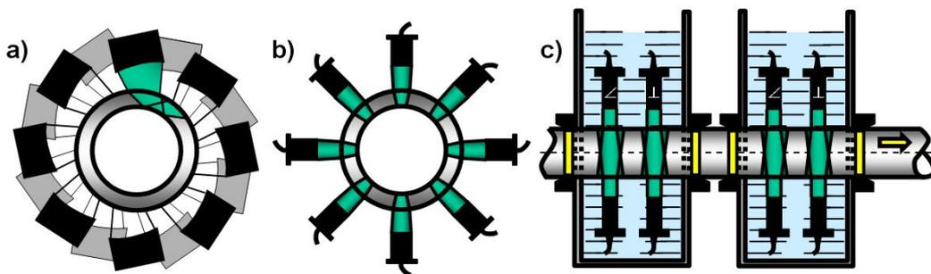
Fig. 1: HRP.R-Echograph high speed tube test a) angle probes for longitudinal defects (only clockwise probes shown), b) probes for wall thickness measurement, and c) test principle with two immersion tanks, each carrying angle and straight-beam probes.
