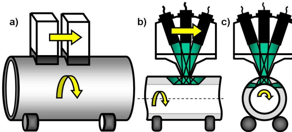
Fig. 3: RPT.R-Echograph rotational tube test with multi-probe holders a) rotation of the tube and linear probe holder movement for helical test traces, b) multi-probe holder in cross sectional view showing transverse defect detection and wall thickness measurement, and c) multi-probe holder showing longitudinal defect detection and wall thickness measurement.
