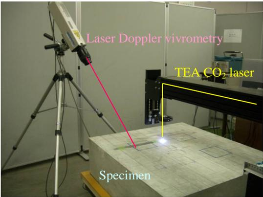
Figure2. Experimental arrangement
