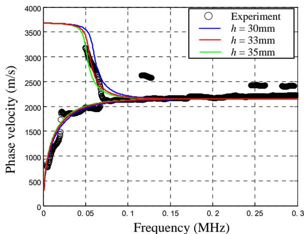
Figure 11. Estimation of depth of defect-A
