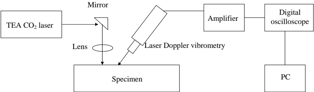
Figure1. Instrumental setup of the experiment
