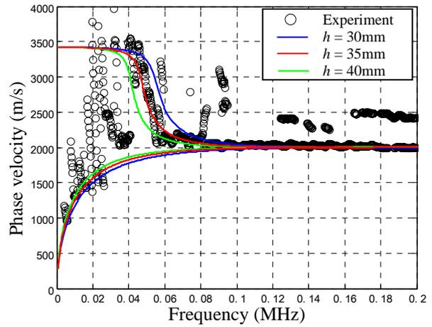
Figure 14. Estimation of depth of crack
