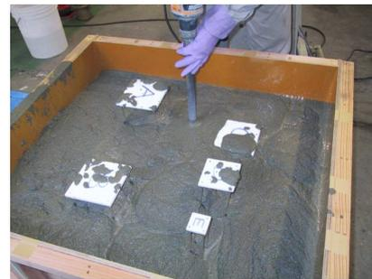
Fabrication of artificial voids
