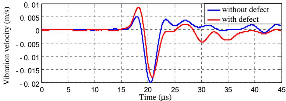
**Figure 6.** Comparison of waveforms between with and without defects
