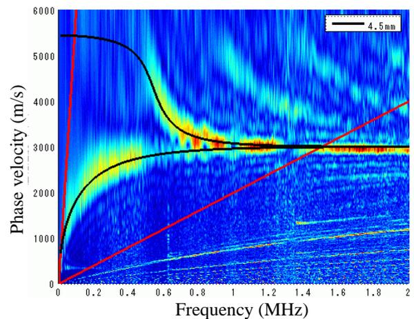
Figure 16. Velocity dispersion curve (after delamination)
