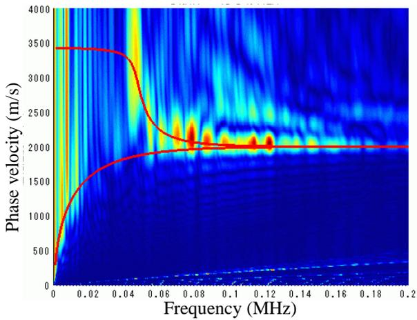
Figure 13. Velocity dispersion curve (cracked specimen)
