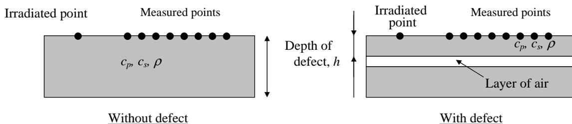
Figure 9. Schematic of analysis model
