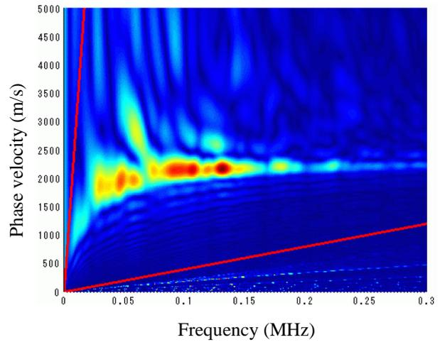
Figure 8. Velocity dispersion curve (defect-A)
