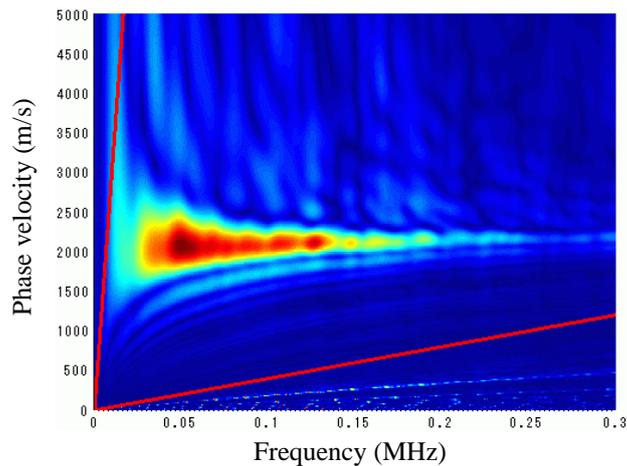
Figure 10. Velocity dispersion curve (without defect)
