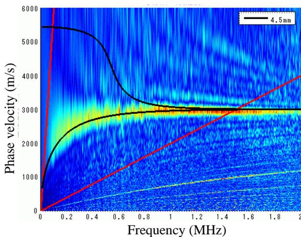
Figure 15. Velocity dispersion curve (before delamination)
