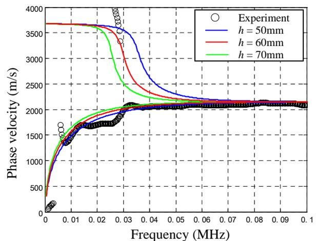
Figure 12. Estimation of depth of defect-B
