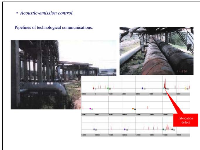
Fig.5 AE-testing of pipeline.
