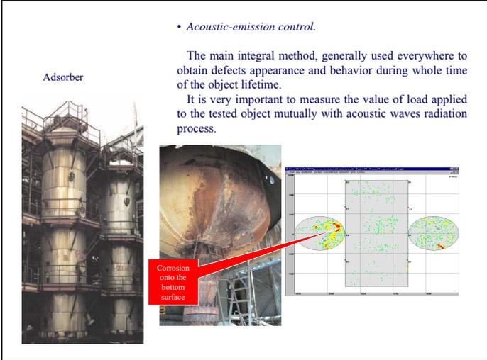
**Fig.3** Determination of defect on adsorber.
