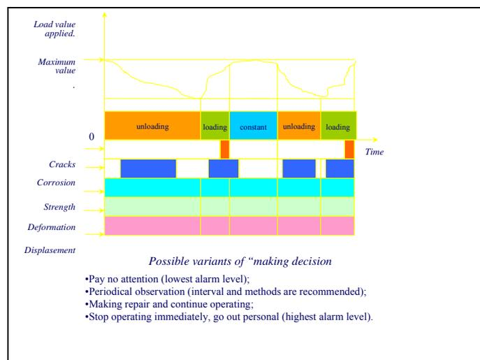
**Fig.10** Defects classifying algorithm principle
