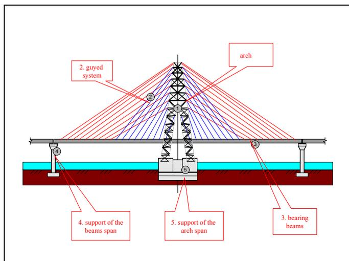
**Fig.9** Monitoring project for guyed bridge construction (Moscow river).
