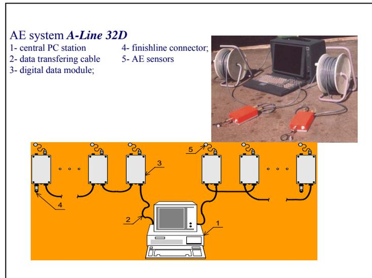
**Fig.1** AE-system A-Line 32D, photo and block diagram.
