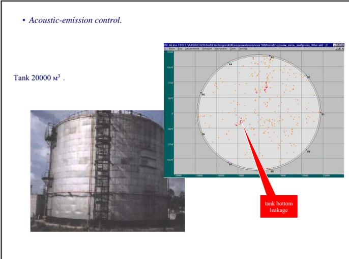
**Fig.4** AE-testing of tank bottom.
