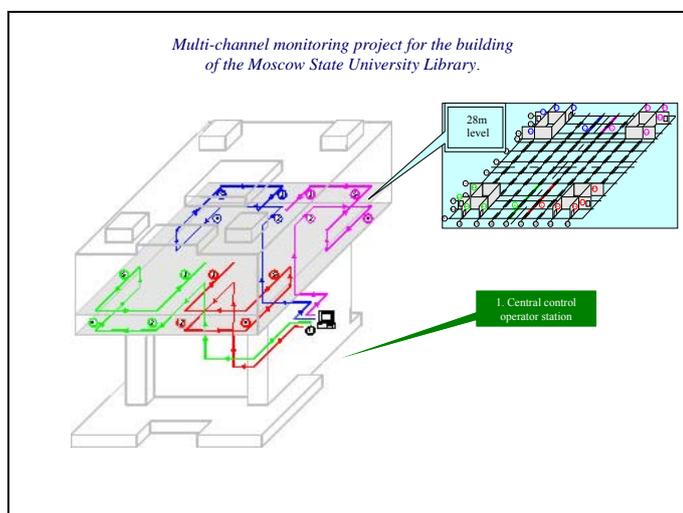
Fig.6 AE-monitoring system for building.
