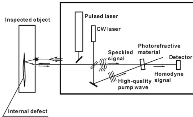
(used as a reference beam) and probe beam illuminating the inspected surface. Forming optical system produces the probe beam focused on the inspected surface. The same optical system collects radiation scattered by the inspected surface. This signal and the pump beam intersect each other in a photorefractive crystal and record a dynamic hologram [4, 5].
