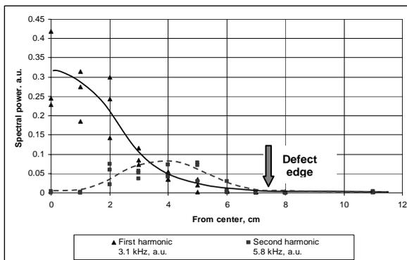
Fig. 11. Sample with the CRACK (depth – 15 mm). Detection accuracy is about 2 cm.
