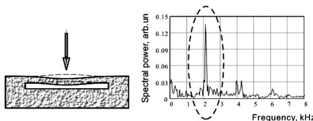
Impact/detection position is over defect.
