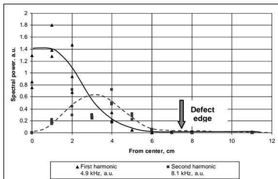
Fig. 12. Sample with the HONEYCOMB defect (depth – 15 mm). Detection accuracy is about 2 cm.
