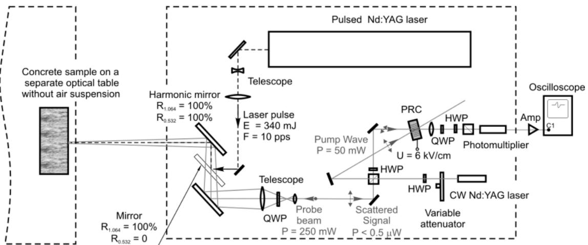
Fig.5. Schematic diagram of laboratory experimental setup.
