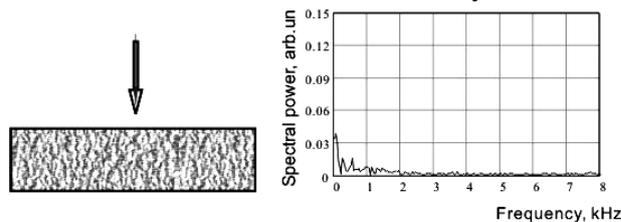
Impact/detection position is over no-defect area.
