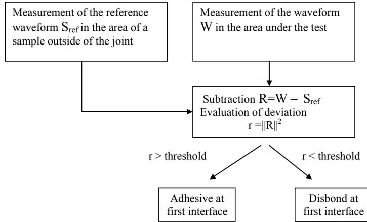
Figure 3. Signal processing algorithm for disbond detection at the first interface.
