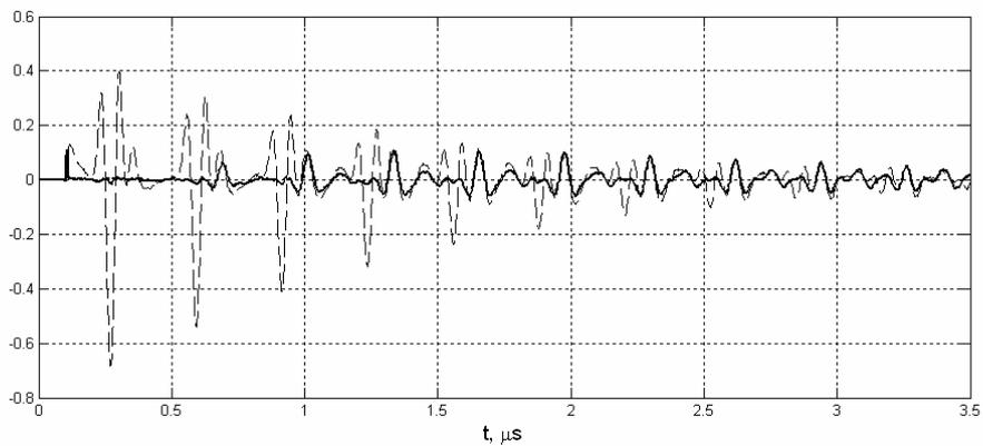
Figure 7. Waveform  $W$  (dashed line),  $W-R_{ref}$  (solid line), obtained for a sample with disbond at the second interface (upper graph), and fully bonded (lower graph). The thicknesses of the adhesive are 0.6 and 0.5 mm.
