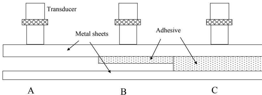
Figure 1. Types of defects: A – disbond at the first interface, B – disbond at the second interface, C – good joint.
