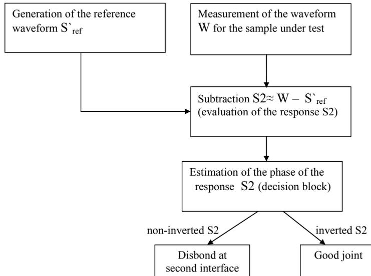
Figure 4. Signal processing algorithm for disbond detection at the second interface
