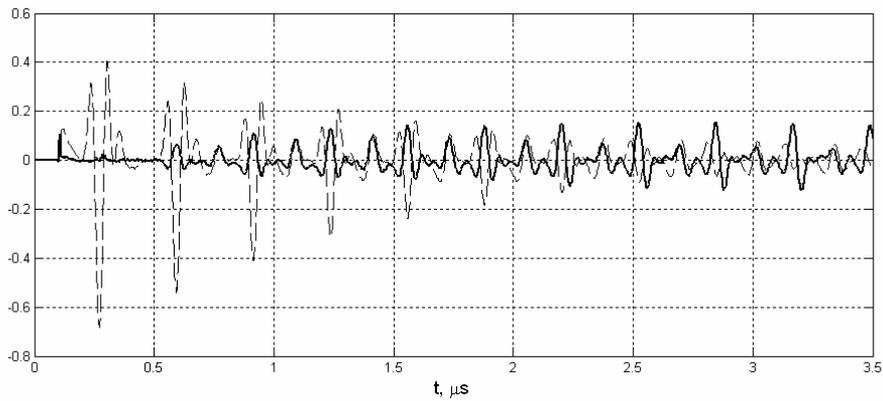
Figure 6. Waveform  $W$  (dashed line),  $W-R_{ref}$  (solid line), obtained for a sample with disbond at the first interface (upper graph), and fully bonded (lower graph). The thickness of the adhesive is 0.6 mm.
