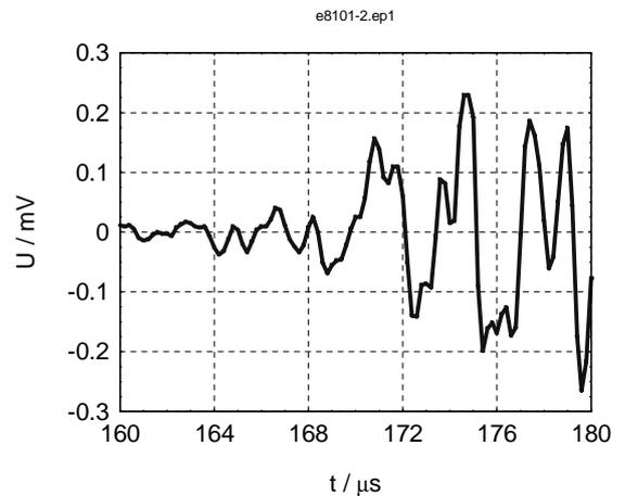
Fig. 9. EME signal time dependence for samples with the slow crack opening (fine structure)
