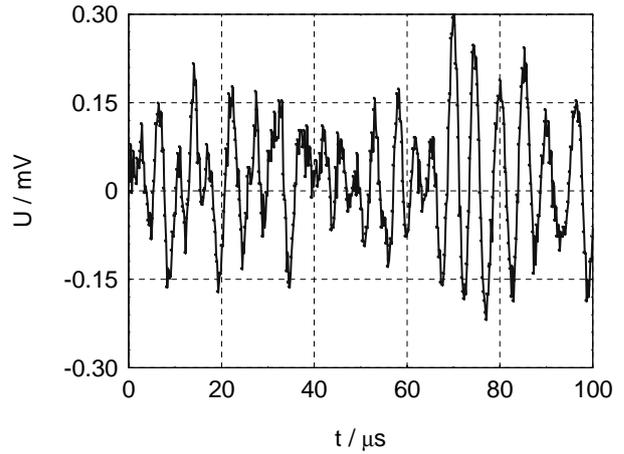
Fig. 7. AE signal in the time domain
