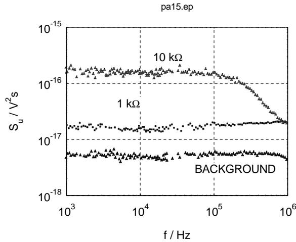
Fig. 4. Noise characteristics of the preamplifier PA15
