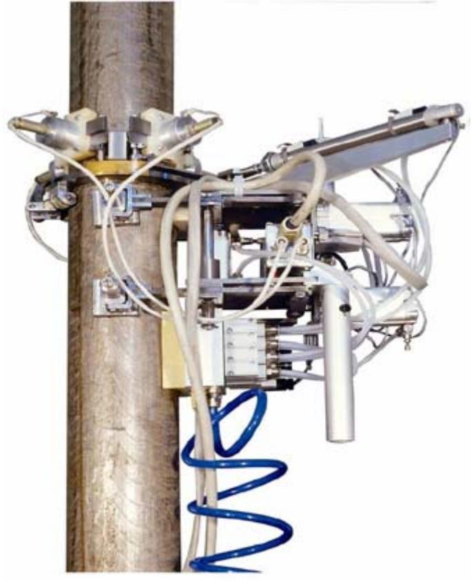
Figure 5. Four probe automated scanner system installed on tested tube.
