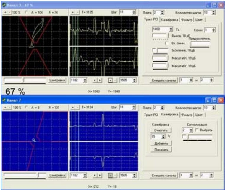
Figure 3. Computer display interface for one eddy current card.
