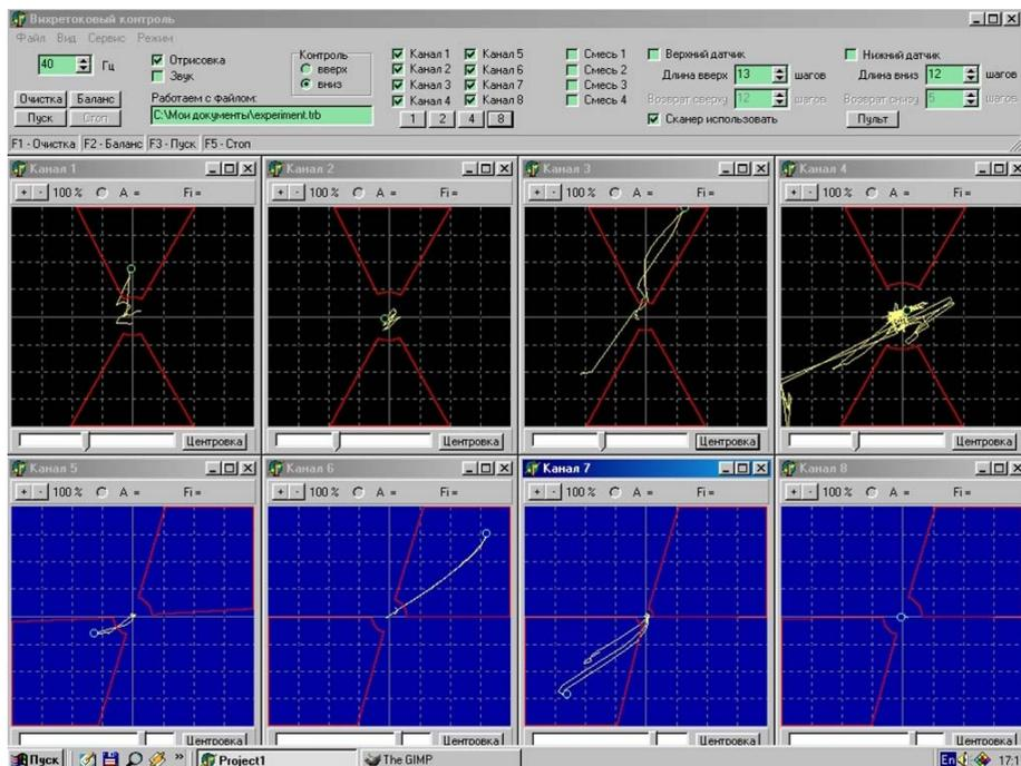
Figure 4. The signal responses obtained from 4 eddy current probes on 2 operational frequencies.
