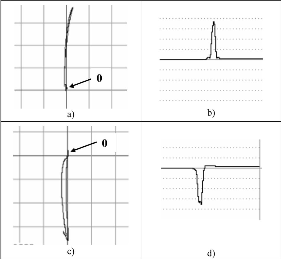
Figure 2. Leotest MDF 3301 eddy current probe signal responses obtained for longitudinal outer surface slots (a, b) and for transverse outer surface slots (c, d).
