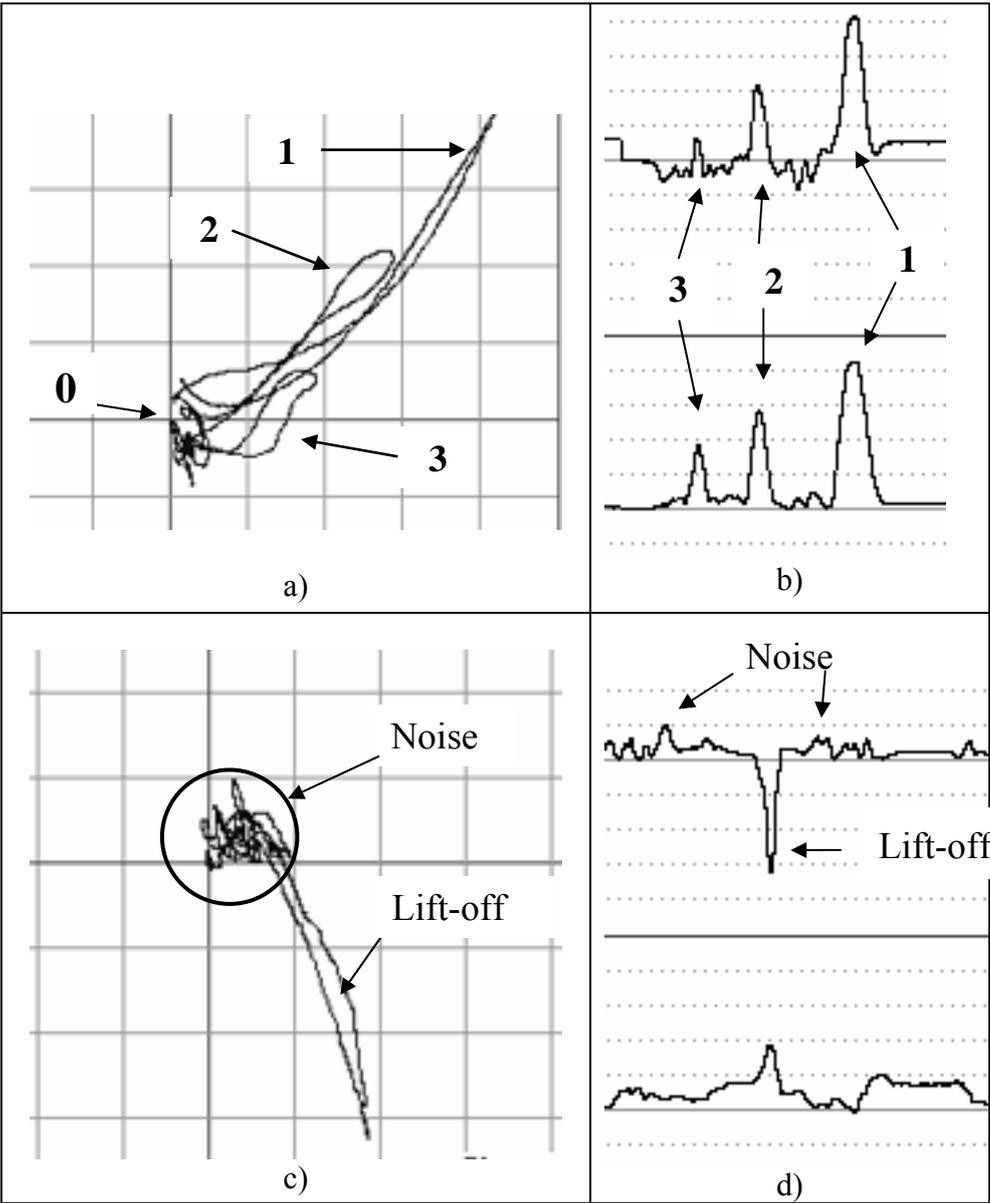
Figure 1. The Leotest 3301 eddy current probe responses obtained for slot with depth of underlying 7,5 mm (1 on a and b); 6,0 (2 on a and b) and 5,0 (3 on a and b) and structural noise and lift-off in complex plane (a, c) and in time sweep mode (b, d).
