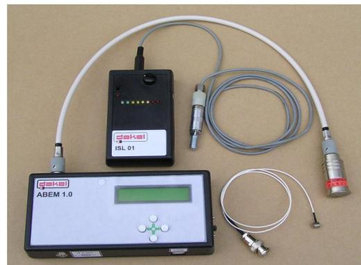
**Fig.12** Examples of tested prototypes of devices for bearings damage identification
