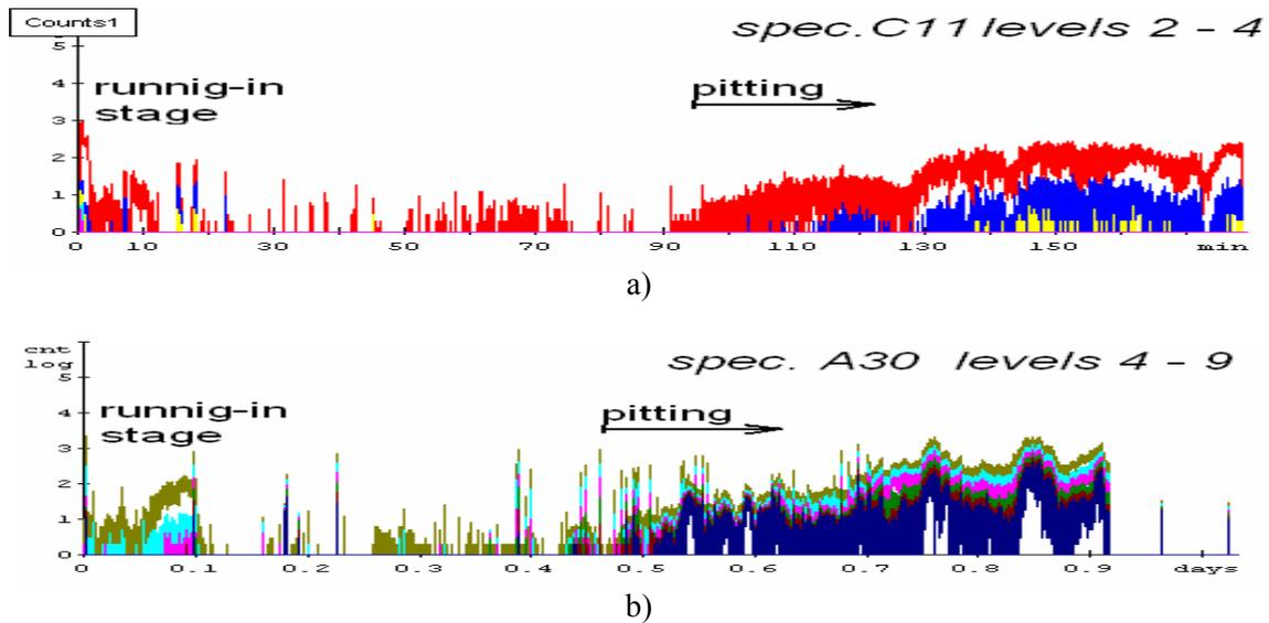
**Fig.6** Numbers of counts overshoots in chosen levels of AE signal a) level 2 to 6 in a grey cast iron sample under high contact load (test time app. 3 hrs), b) level 4 – 9 in carbon steel samples (test time app.22 hrs.)
