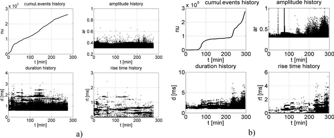
**Fig.9** Overview of basic AE events parameters treatment – cumulative number, amplitude, duration and rise time history for grey cast iron (a) and for carbon steel (b).
