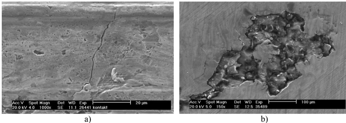
**Fig.1** Micrographs of short crack in contact fatigue trace (cast iron a) and developed pitting in carbon steel b)
