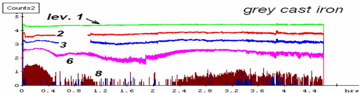
**Fig.5** Number of overshoots (counts rate) in measured levels of AE signal in the course of test - example of various measured levels with low energy (grey cast iron). Level 8 will be used for identification of stages.
