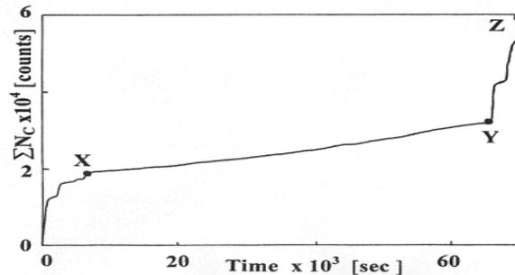
**Fig.4** Example of summation record of number of AE overshoots (counts) in the course of contact fatigue test of grey cast iron.
