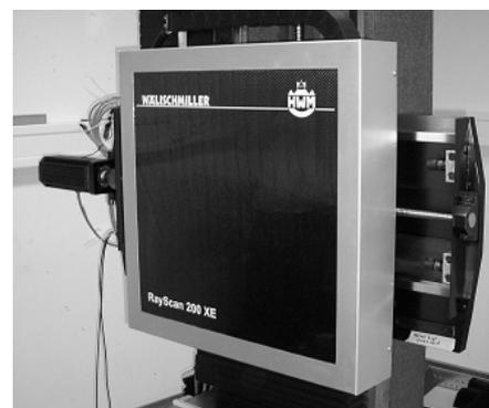
Fig. 2. X-ray detector PerkinElmer RID 1640 ALI ES of the CT Rayscan 250 E
