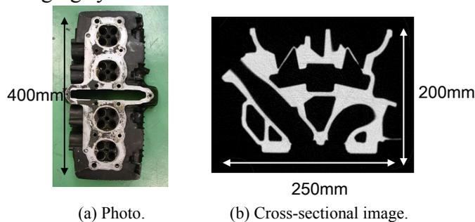
Fig.5 Application of the system to a motorcycle cylinder head.
