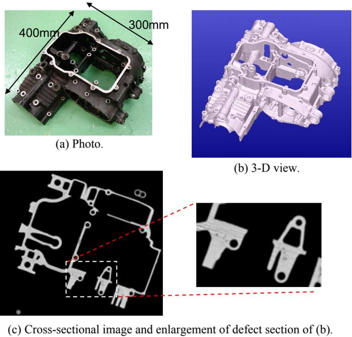
Fig.6 Application of the system to a motorcycle engine cover.
