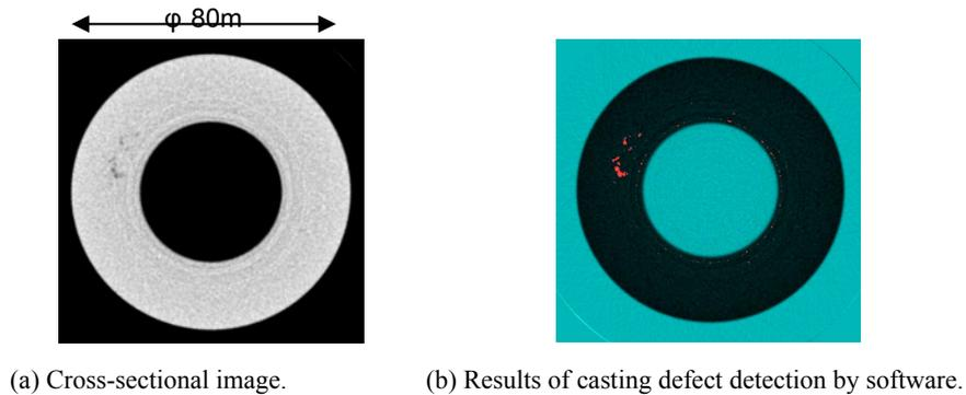
Fig.7 Example of casting defect detection by software.
