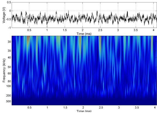
**Figure 3.** CWT of a series of AE pulses generated by the transformer
