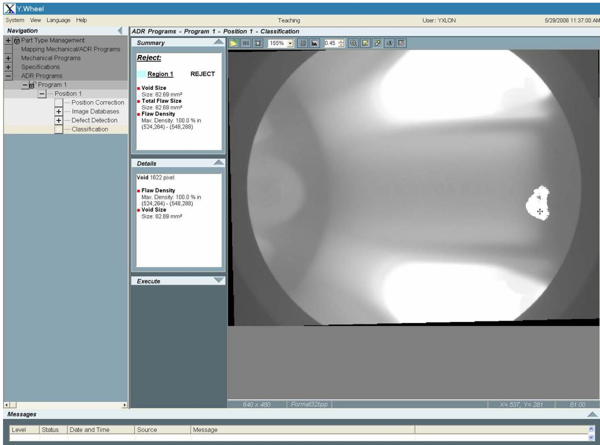
**Figure 4.** Use of software building blocks: dynamically generated view for testing the classification.
