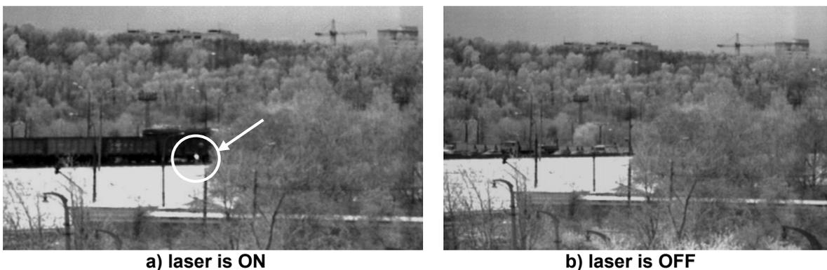
Fig. 1. Detection of sniper sight of PO4x34 type (distance 500 m) with the help of «SPIN-2» instrument
