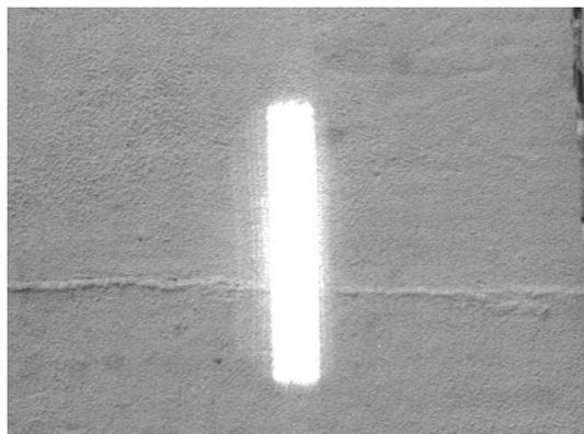
Fig. 3. Laser illumination pattern shape at distance 30m
