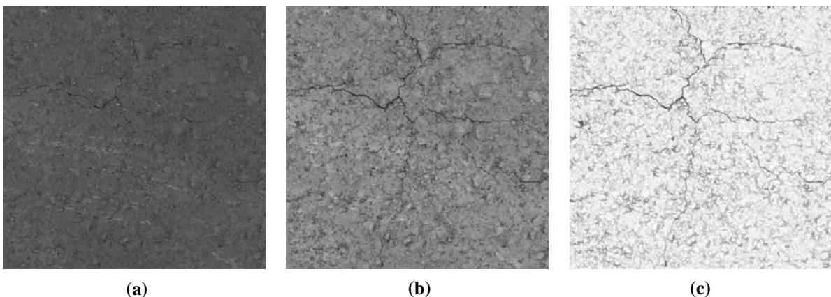
**Fig. 1** Results of pre-processing: (a) Original image (b) Image after erosion and reduction of resolution (c) Image after background subtraction
