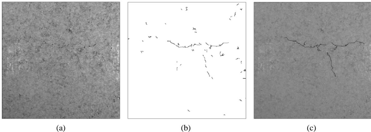
**Fig. 5** Brick with significant cracks (a) Original image (b) Crack image before tracing-algorithm (c) Original image with detected cracks overlaid
