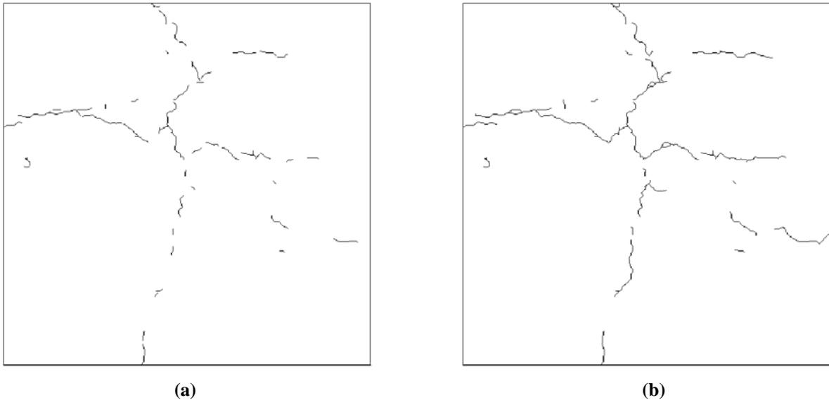
**Fig. 3** Linking of crack parts during tracing-algorithm: (a) Initial binary image (b) Resulting crack image
