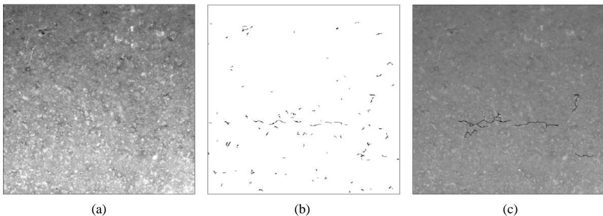
**Fig. 6** Brick with weak cracks (a) Original image (b) Crack image before tracing-algorithm (c) Original image with detected cracks overlaid
