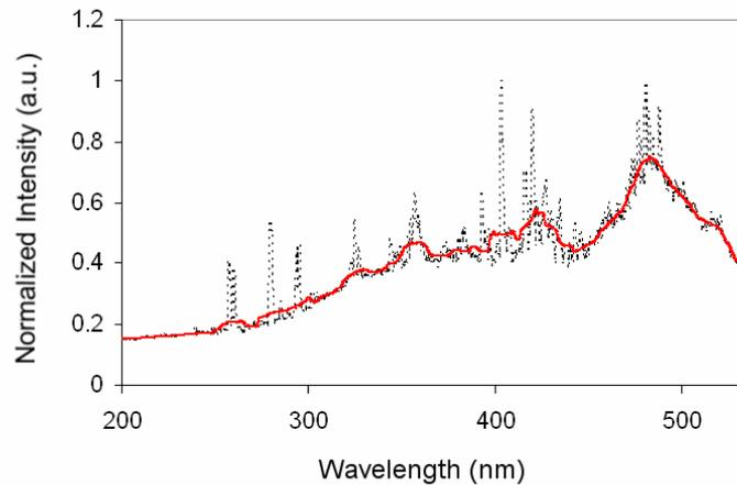
b) TIG spectra with embedded fiber
