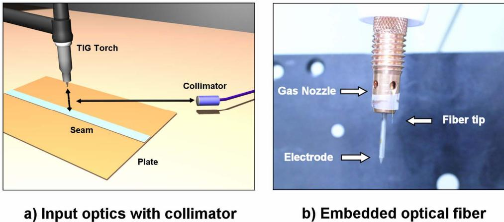
Figure 1. Input optics with collimator scheme and image of the fiber embedded into the TIG torch.
