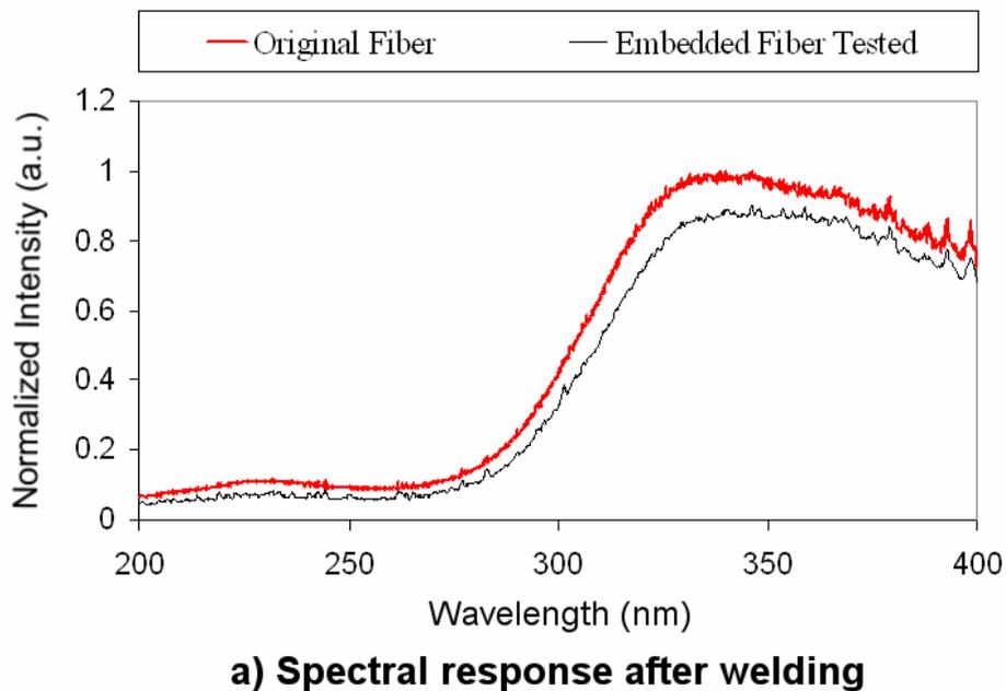
Figure 2. Spectral response of the fiber before and after extensive welding tests.
