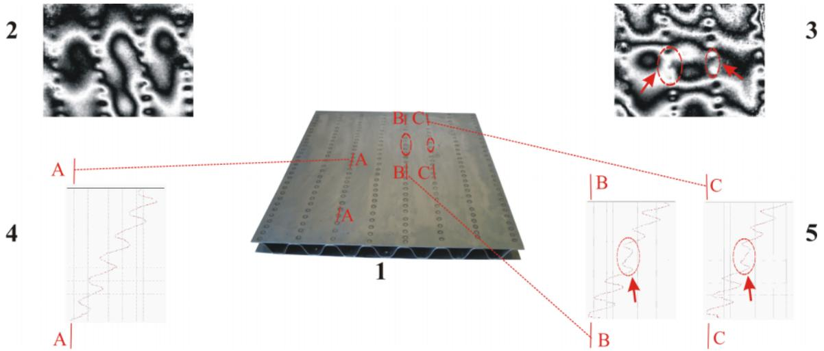
**Figure 3.** Results of quality control of a three-layer made by a spot resistance welding (for designation see Figure 2)
