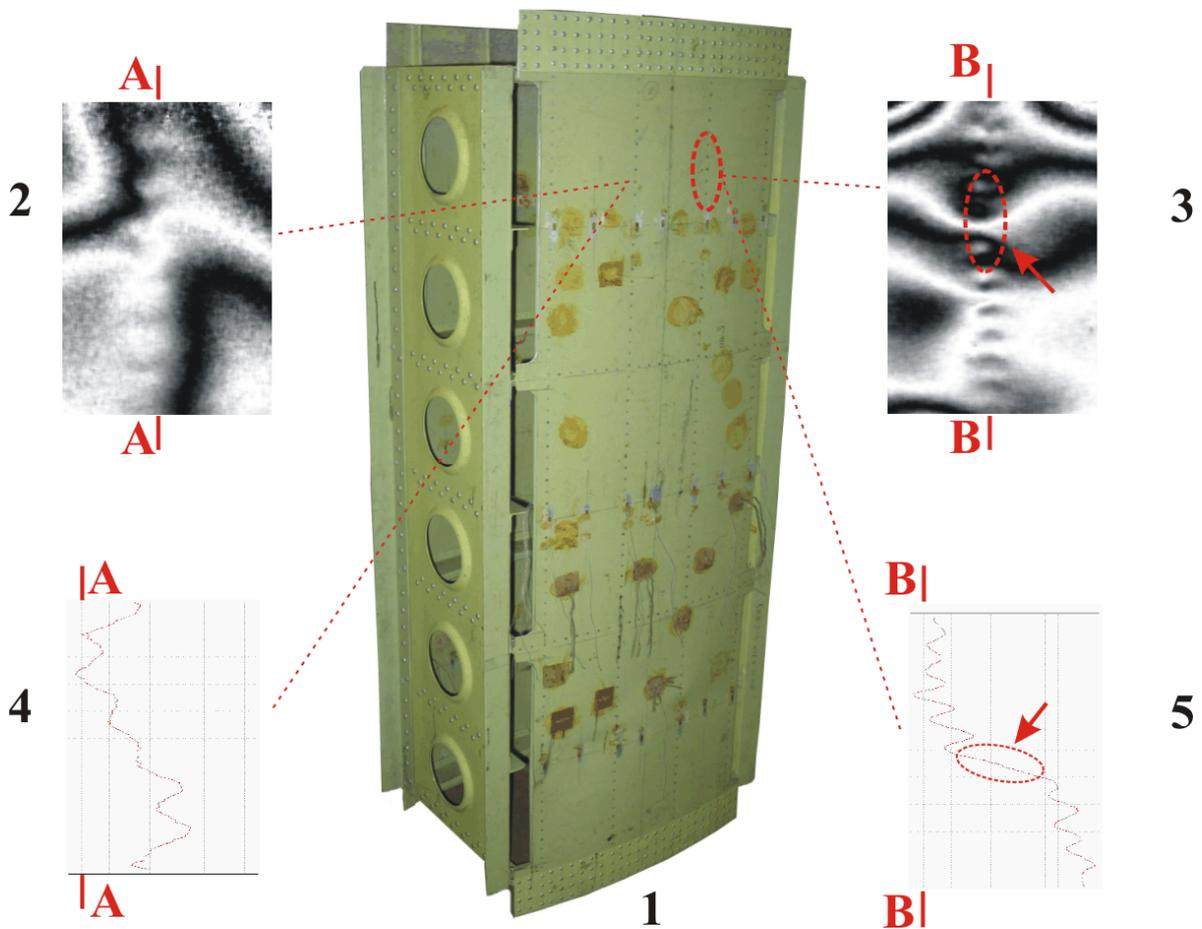
**Figure 4.** Results of quality control of thin-walled structures (for designations see Figure 2)
