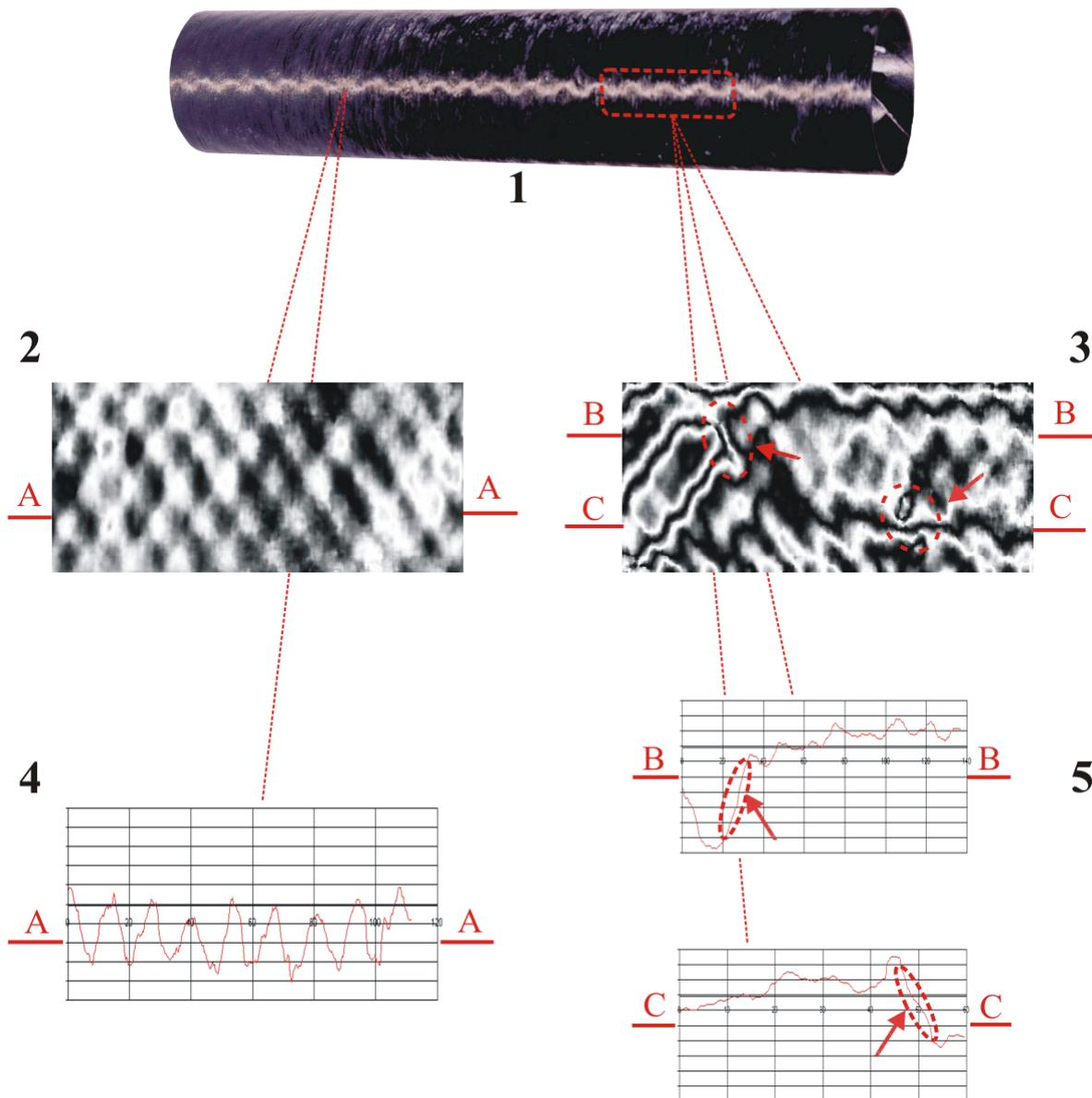
**Figure 2.** Results of quality control of glass-reinforced plastic tubular element: 1 – general view; 2,3 – typical interference pattern obtained in testing areas, respectively, with and without defects; 4,5 – change in derivative from out-of-plane displacements of structures along the selected sections (zones of defects are distinguishes and shown by arrows)
