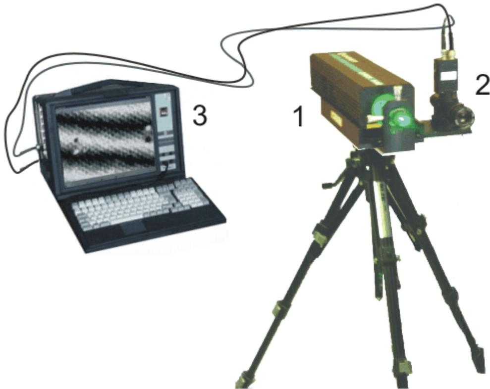
**Figure 1.** General view of a shearographic unit: 1 – laser, 2 – shearographic module; 3 – computer.
