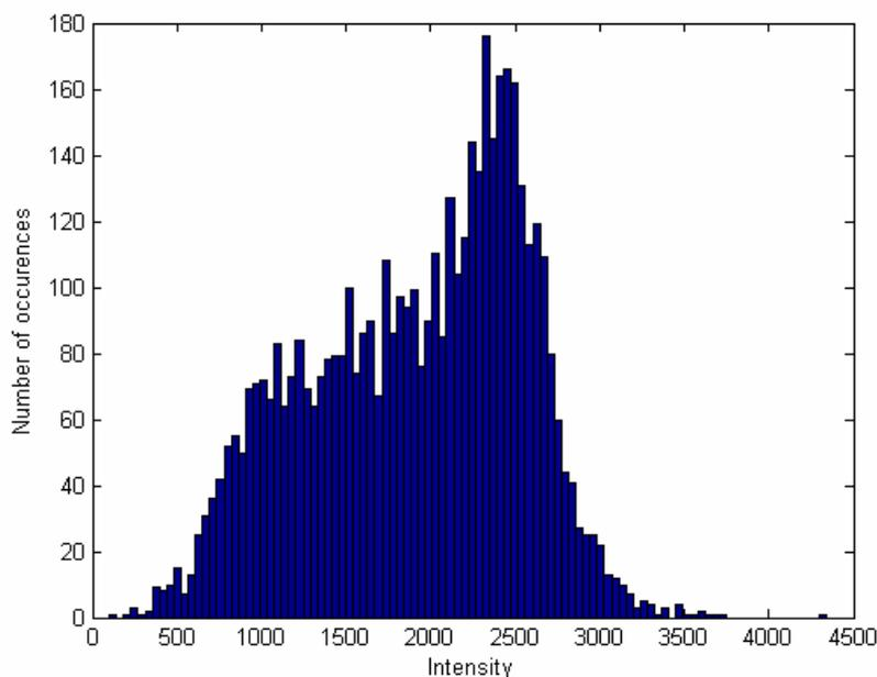
Figure 6: Histogram of the difference of two images of a heater with defects and a pulse time of 0.3 s
