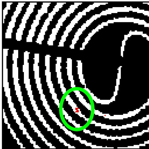
Figure 7: Defects in a heater excited with a pulse of 0.2 s
