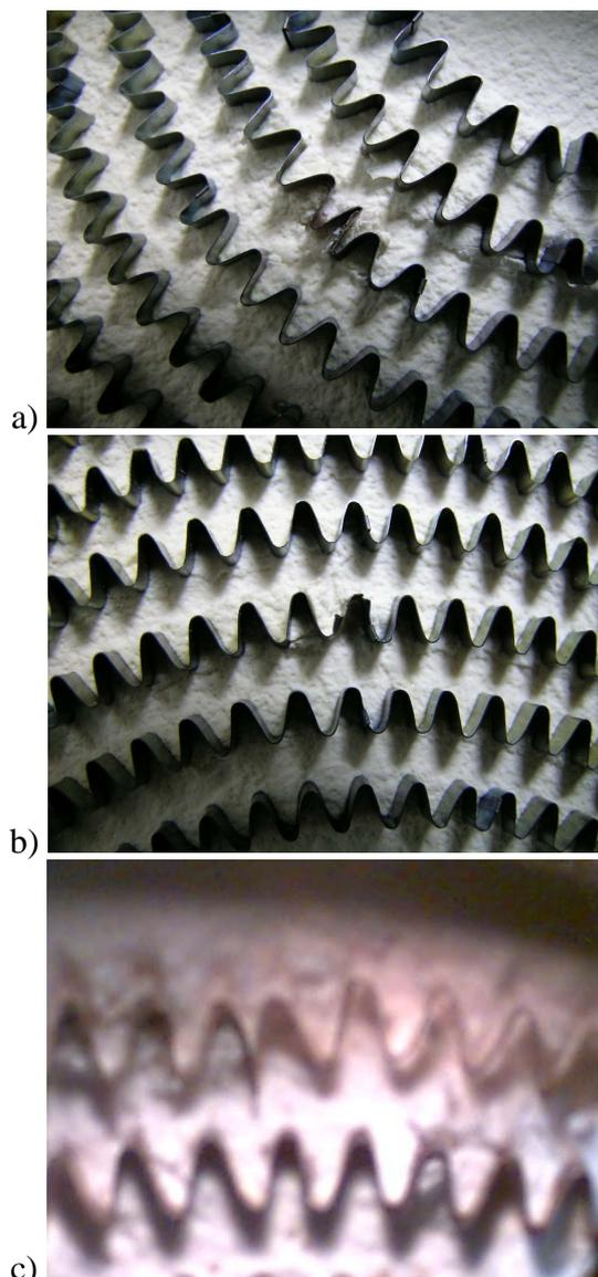
Figure 1. Real and artificial defects on radiant heaters: a) Excess of material as a consequence of a link. b) Lack of material as a consequence of a cut on the surface of the wire. c) Parts of the wire that are not in contact with the substrate.
