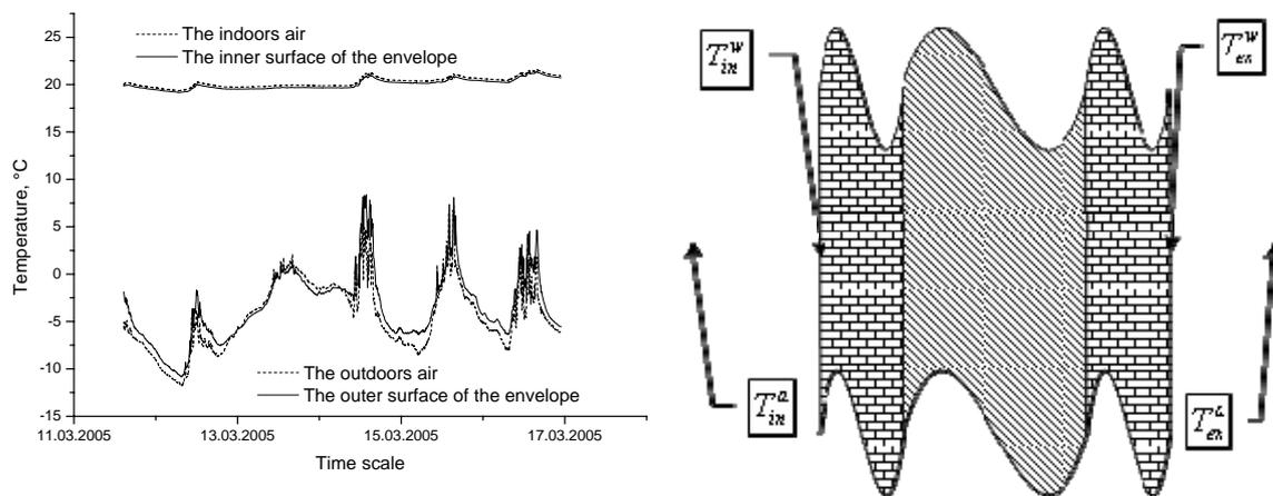
Fig. 2. Typical temperature time series of the reference zone (left). Sensor position at the reference zone (right).
