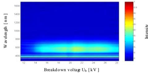
**Figure 5.** The influence of the supplying voltage value in the point-point spark gap in air on the length of the light wave emitted
