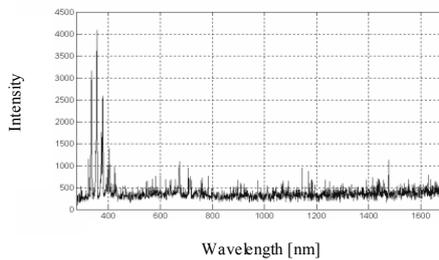
**Figure 3.** Optical spectrum of partial discharges generated in the point – point system in air, at the voltage of  $0.5U_b$
