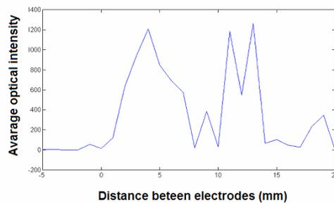
**Figure 12.** Dependence of the average optical intensity on the distance between the electrodes in the band 270-1700 nm.
