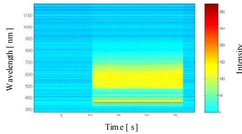
**Figure 6.** Changes of the optical spectrum during the arc burning time of the disruptive discharge in the point-point spark gap in air
