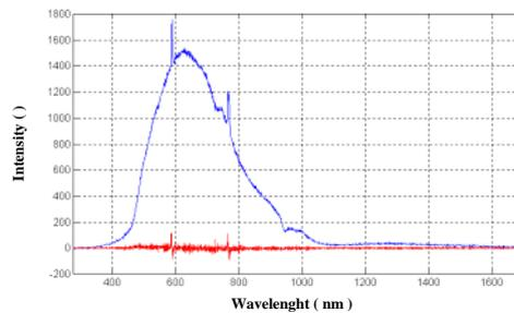
**Figure 10.** Optical spectrum of creeping discharges in air in the range from 270 to 1700 nm
