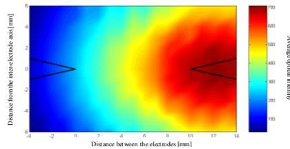
**Figure 7.** Optical spectrum distribution in a point tangent to the surface of the spark-gap points for discharges of the point-point type in air
