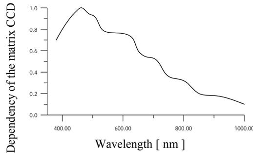
**Figure 2.** Dependency of the spectrometer matrix sensitivity on the radiation wave length
