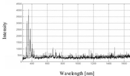
**Figure 4.** Optical spectrum of partial discharges generated in the point – point system in air, at the voltage of  $0.8U_b$
