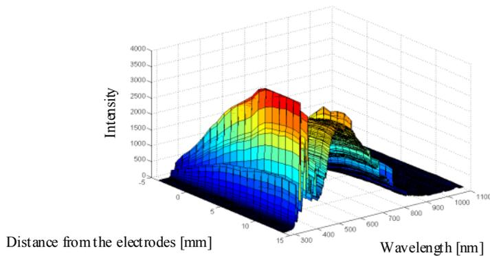
**Figure 8.** Optical spectrum distribution on the inter-electrode axis for a point-point spark-gap in air
