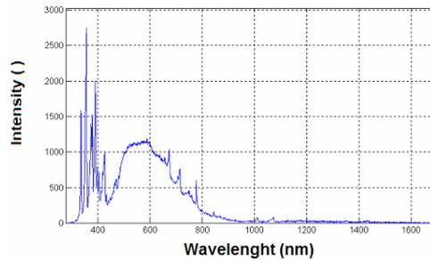
**Figure 9.** Optical spectrum of disruptive discharges in the point-point system in the wavelength range 270-1700 nm
