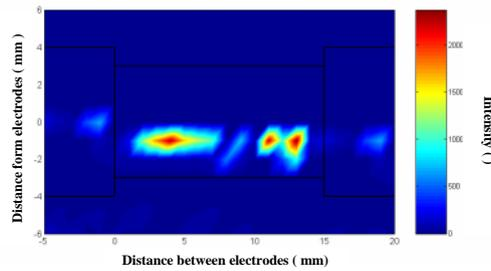
**Figure 11.** Distribution of the average optical intensity in the interelectrode space in the band 270-1700 nm
