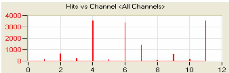
Fig.6 large increment of AE hit for channel 4 and 6 ( leakage occurrence)
