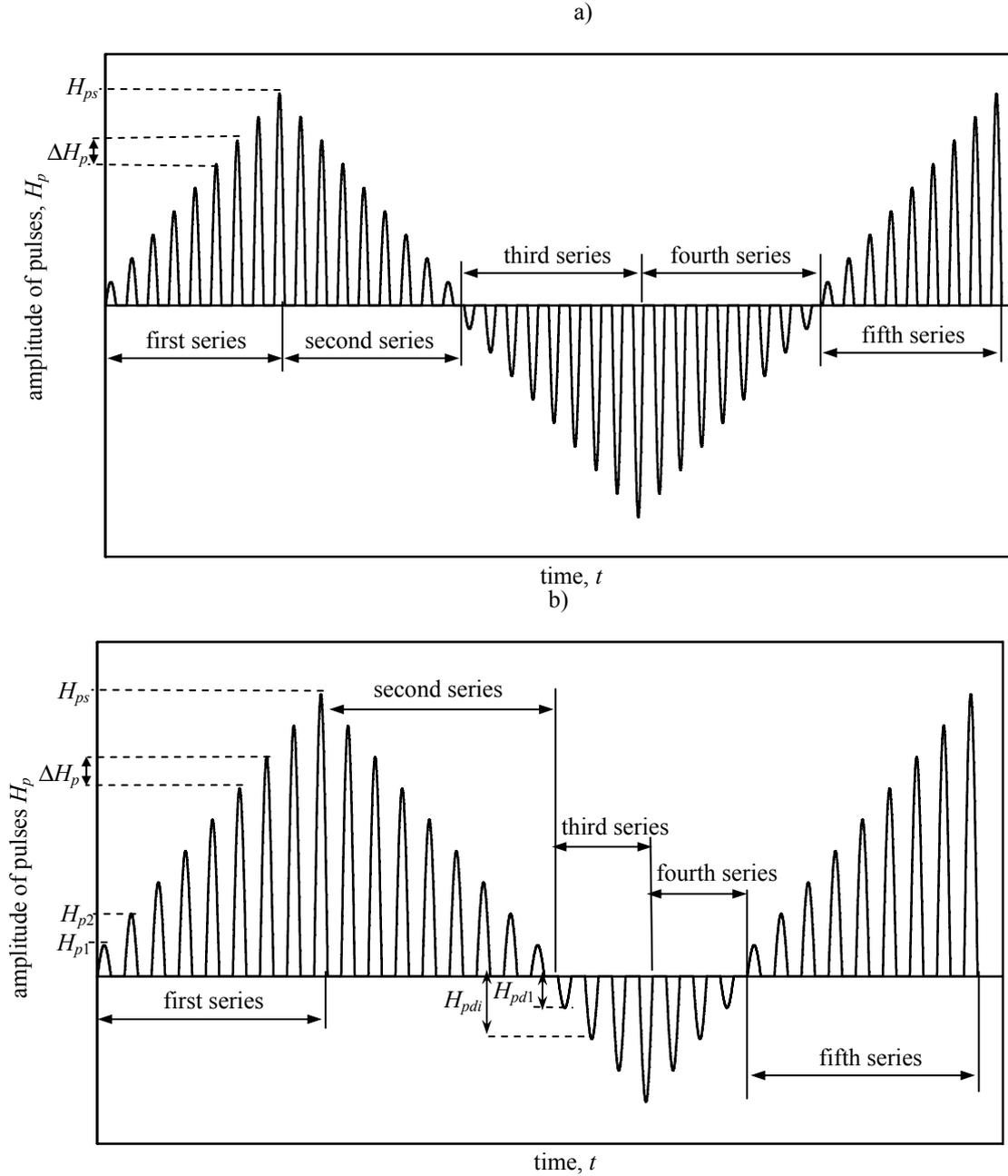
Figure 1. Variation of the amplitude of magnetizing pulses in time for receiving the curve of the gradient of normal component of residual-magnetization field strength or its hysteresis loop (a) and return curve (b)
