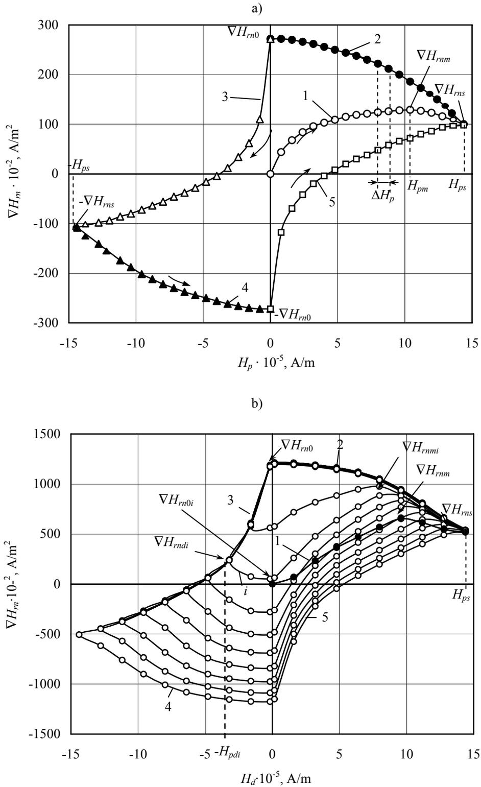
Figure 2. Normal magnetization curve (1) of the gradient of the normal component of the residual magnetization field, of branches (2, 3, 4, 5) of its hysteresis loop (a) and the return curves (b)
