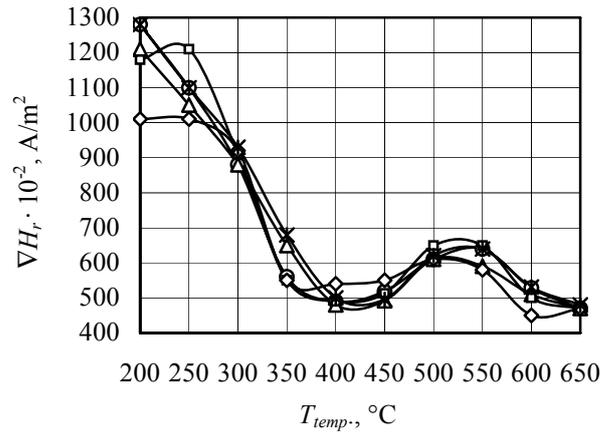
Figure 3. Gradient of normal component of residual magnetization field strength of the silicon steel in dependence on tempering temperature at the quenching temperatures:
