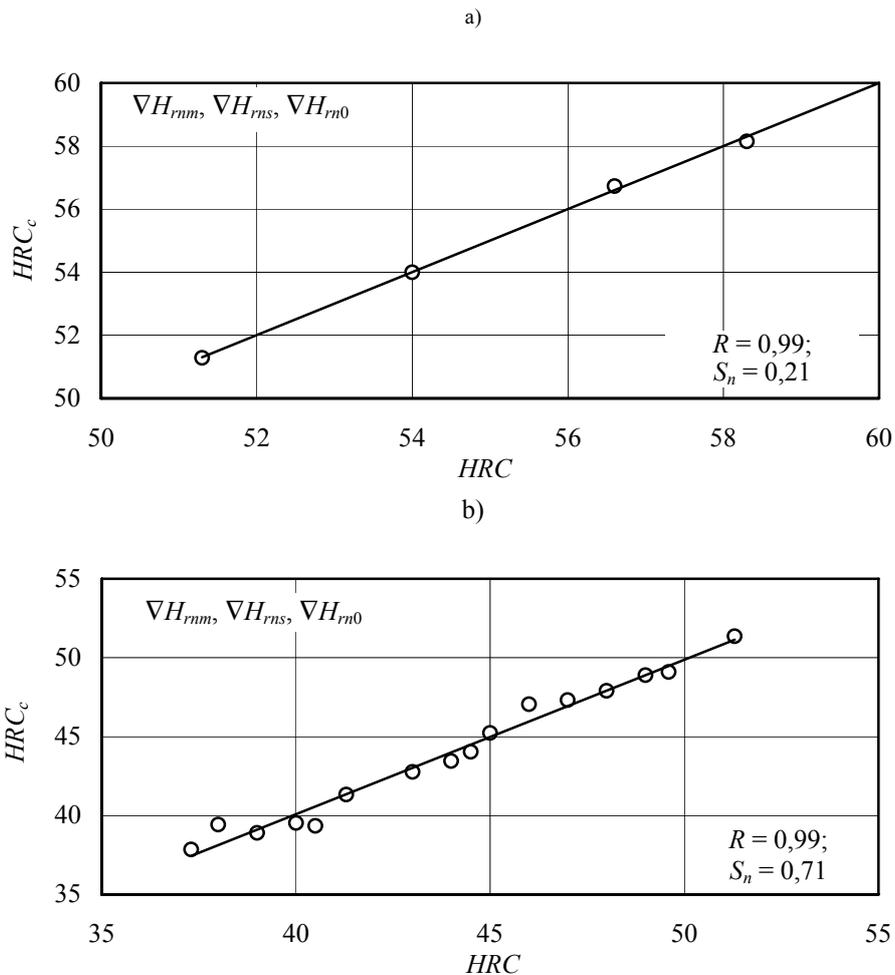
Figure 5. Correlation between the hardness  $HRC$ , measured by Rockwell, and the hardness  $HRC_c$ , calculated using three parameters at testing the low-temperature (0–300 °C) tempering of the steel 50XГФА (a), and using the same parameters for the range of 300–600 °C (b).
