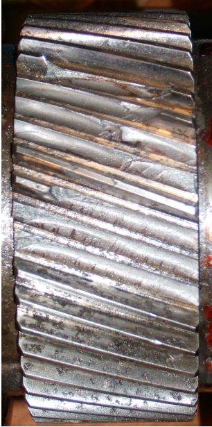
Fig. 6. Gear wheel after a damage
