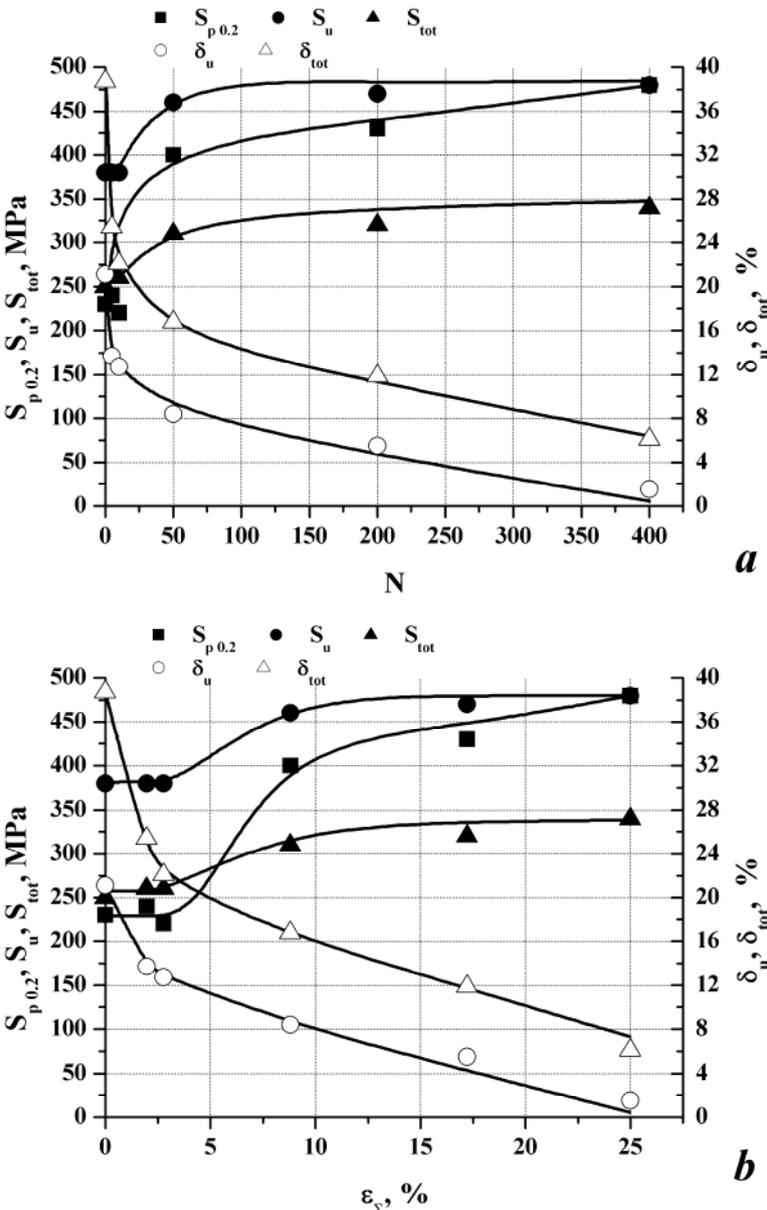
Fig. 3. The variation of residual mechanical properties under tensile testing depending on the number of cycles (a) and accumulated plastic deformation (b) of the steel under study.
