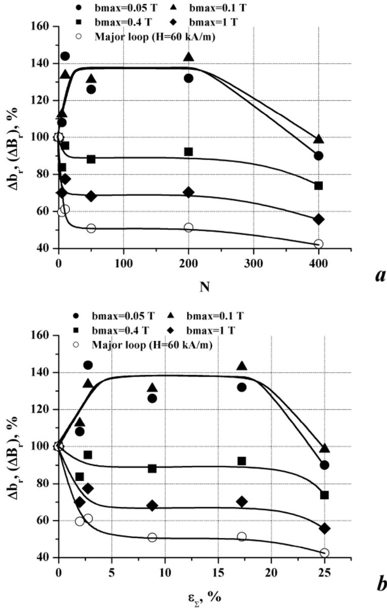
Fig. 2. Relative change of residual magnetic induction as dependent on the number of cycles (a) and accumulated plastic deformation (b) of the steel. The values of residual magnetic induction for the steel under annealed initial condition are taken to be 100% (see the table).
