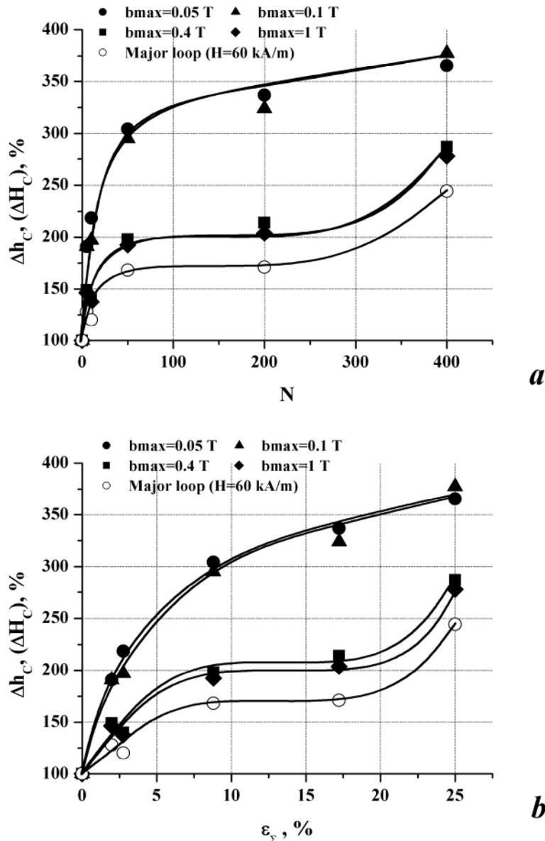
Fig. 1. Relative change of the coercive force as dependent on the number of cycles (a) and accumulated plastic deformation (b) for the steel under study. Coercive force values for the steel under annealed initial condition are taken to be 100% (see the table).
