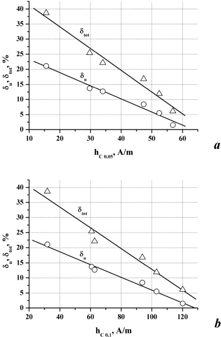
Fig. 4. Relationships between the variation of the plasticity characteristics and the magnetic characteristics of the steel under study.
