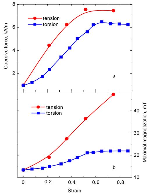
Fig. 5. The effect of deformation in tension and in torsion on the coercive force (a) and maximal magnetization (b) of steel 03G21Kh13
