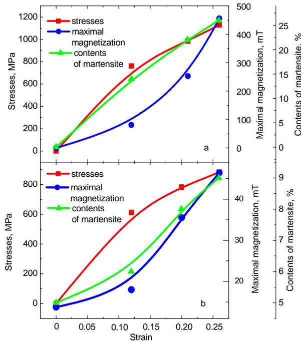
Fig. 6. Stress-strain curves, deformation dependences of maximal magnetization and contents of strain-induced martensite for steels 05G20S2 (a) and 03G21Kh13 (b)
