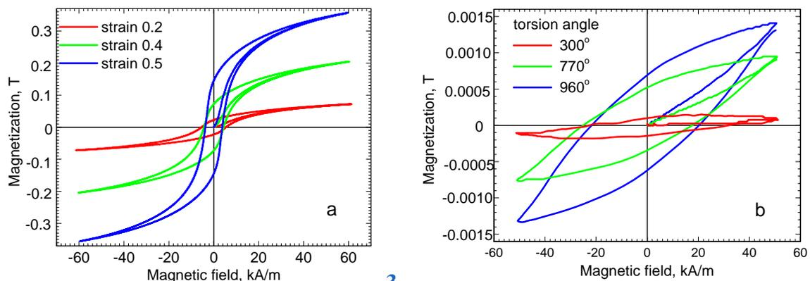
more  $\alpha'$ -martensite is formed in the specimen bulk in tension, than in torsion. This is attributable to the nonuniform distribution of shearing strain in the specimen cross section in torsion tests (there is no deformation in the central part, whereas on the specimen surface deformation attains maximal values).
