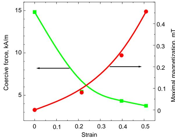
Fig. 3. The effect of tensile strain on the magnetic characteristics of steel 05G20S2
