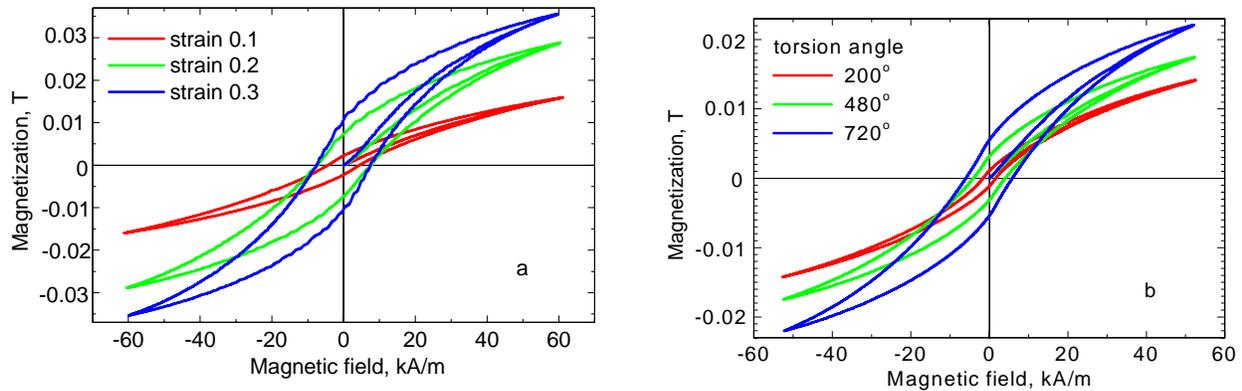
Fig. 4. Magnetic hysteresis loops for steel 03G21Kh13 in tension (a) and in torsion (b)
