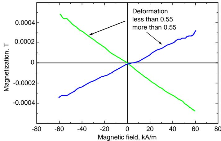
Fig. 1. Magnetization reversal curves for steel 30G21Kh13
