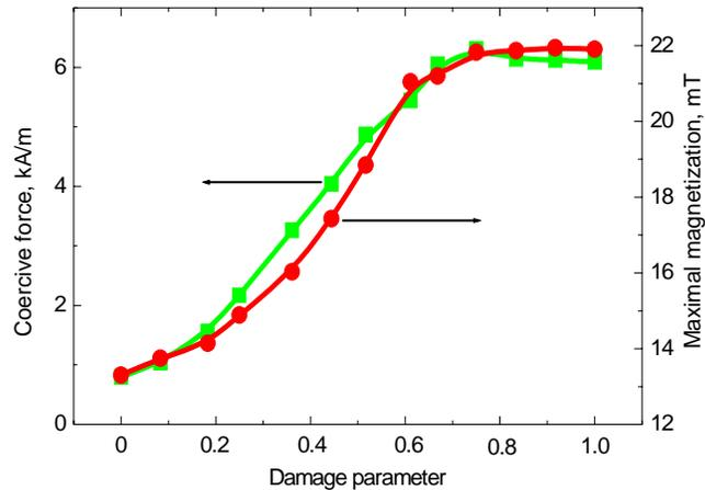
Fig. 7. Magnetic characteristics of steel 05G21Kh13 as functions of the damage parameter in torsion
