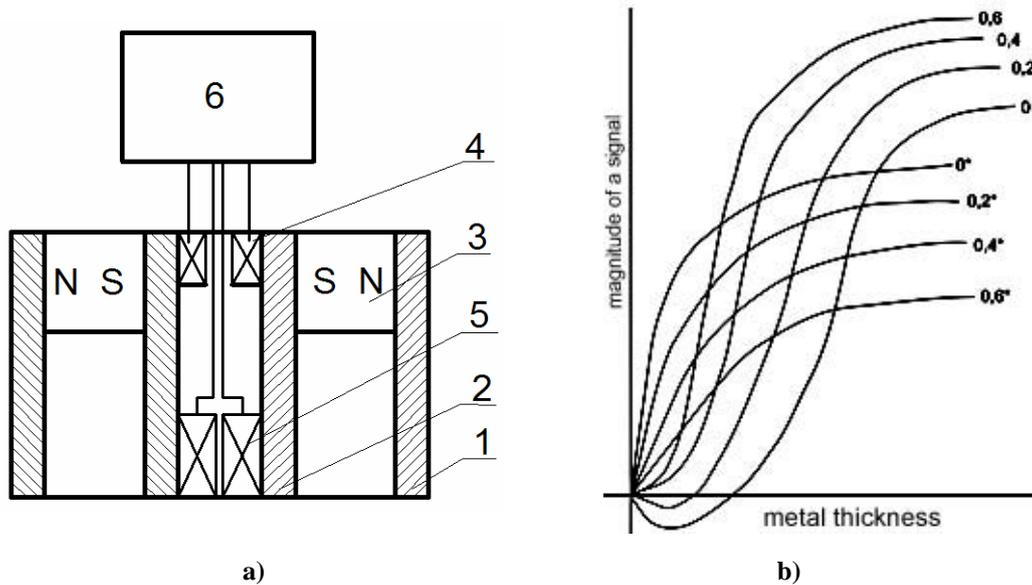
**Fig. 2.** The transducer (based on permanent magnets) for simultaneous measuring the thickness of magnetic base and nonmagnetic coating on it:
