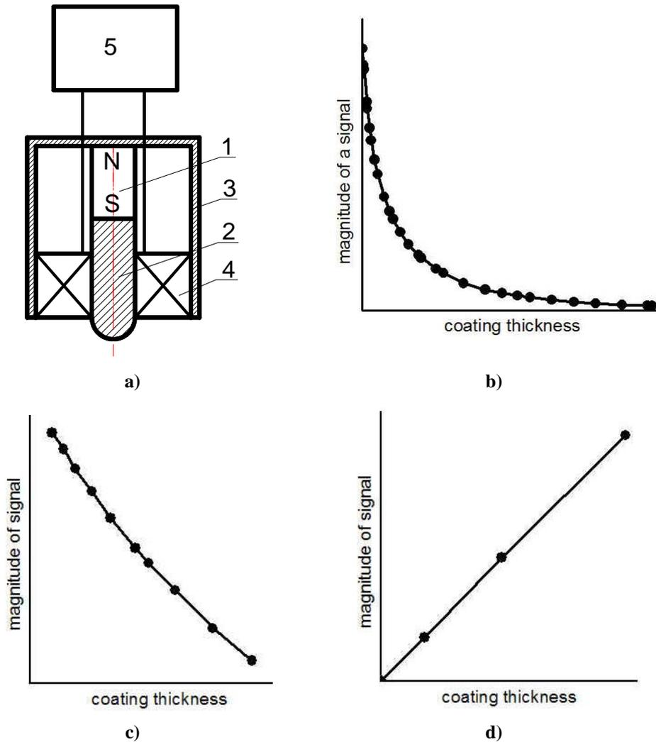
**Fig. 1.** The transducer (based on a permanent magnet) for coating measurements: **a)** the scheme of the transducer; **b)** the dependence of signal for the thickness of nonmagnetic coating on steel base; **c)** the same for the thickness of nickel coating on steel base; **d)** the same for the thickness of nickel coating on nonmagnetic base.
