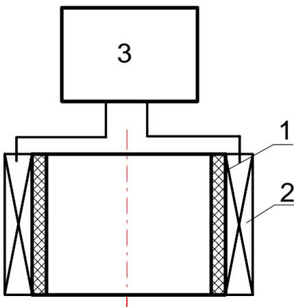
**Fig. 4.** The transducer for residual magnetization measuring
