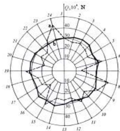
Fig. 5. Distribution of forces in studs at the check:
