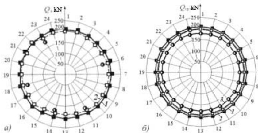
Fig. 6. Results of acoustic strain measurement: distribution of forces  $Q$  in studs (a) and mean forces  $Q_{cp}$  in connection (b) at different phases: 1 - assembly, 2 - recheck after hydro-pneumatic tests, 3 - torque retention loss (actual forces) (1 ... 24 - numbers of studs)
