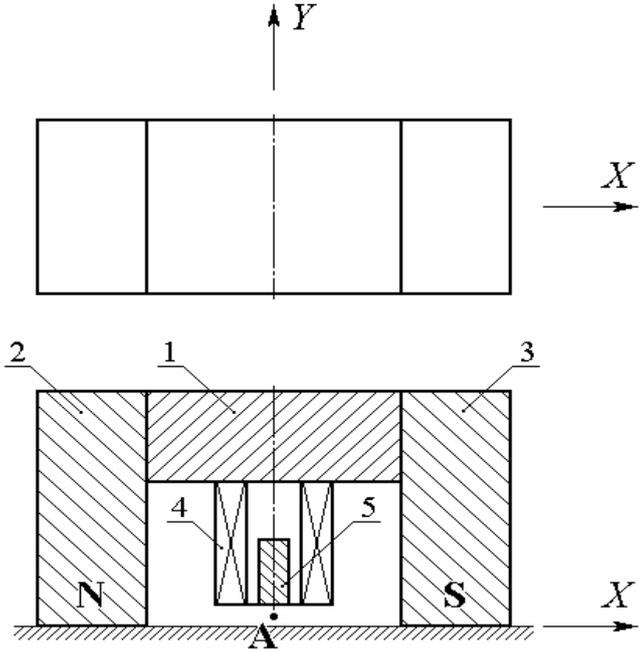
1 - constant magnet, 2 and 3 - pole tips, 4 - measuring coil, 5 - core
