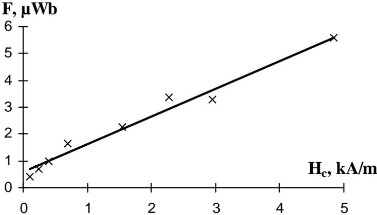
Fig. 2. Dependence of the magnetic flow  $F$  from coercive force  $H_c$ .
