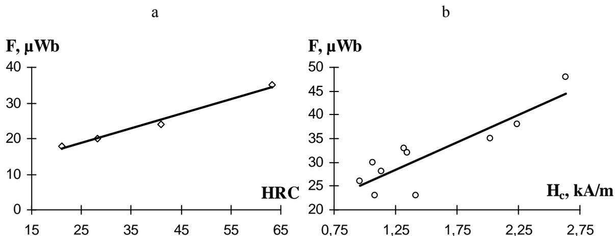
Fig. 3. Dependence of the magnetic flow  $F$  from hardness HRC (fig. 3a) and coercive force (fig. 3b)
