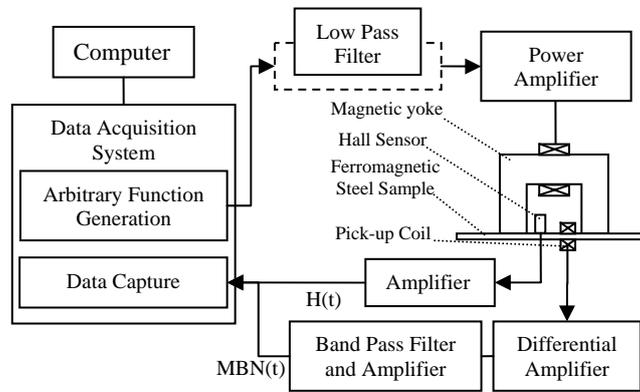
**Figure 3.** Schematic diagram of experimental setup for MBN measurements.
