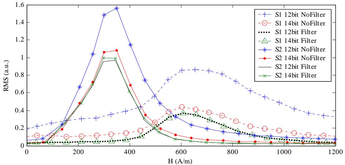
**Figure 4.** RMS profiles of the MBN signal obtained with cold rolled (S1) and cold rolled and annealed (S2) samples with 12-bit and 14-bit resolution unfiltered and filtered trapezoidal waveforms.
