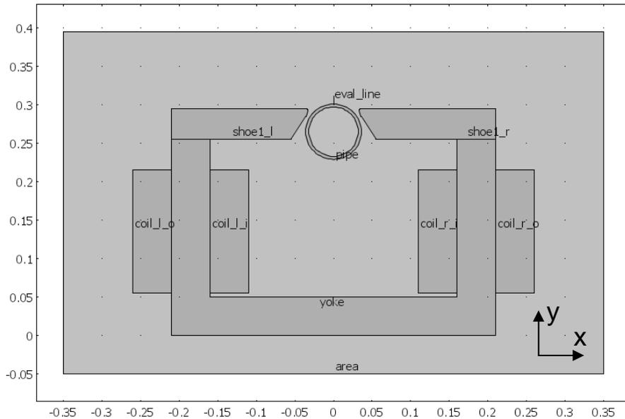
**Figure 1:** sketch of the setup used for the simulations. All measures are in meters.
