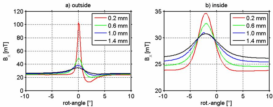
**Figure 8:** comparison of an inside and outside tilted notch: the notch size is 0.1 x 1.5 mm (width x depth) large and tilted at an angle of 60°. Subfigure a) and b) show MFL signals for the outside and inside case respectively for different values of lift-off.
