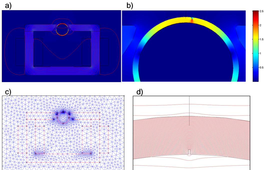
**Figure 2:** examples of simulation results: a) complete setup with flux lines. b) detail of a) showing an oblique outside notch at  $10^\circ$  position, the color-code gives the normalized B-field. c) view of the automatically generated mesh. Subfigure d) is a detailed view of flux lines around an inside notch.
