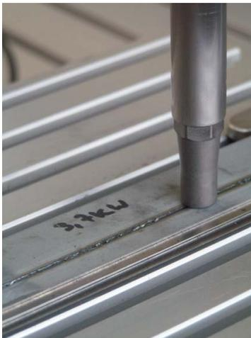
Fig. 1: Eddy current probe on laser welding seam
