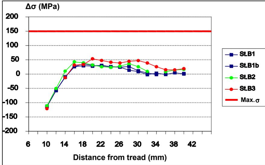
Fig.2 – Operated wheel. The compressive stresses are compensated at about 15 mm from the tread
