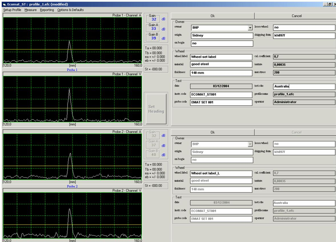
Fig.6 – User interface of BHP-Billiton system: two EMAT units can jointly operate to test a wheelset
