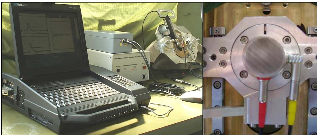
Fig.3 – Ecomat-ST: portable manipulator and dual sensor EMAT probe for shear waves of cross polarization
