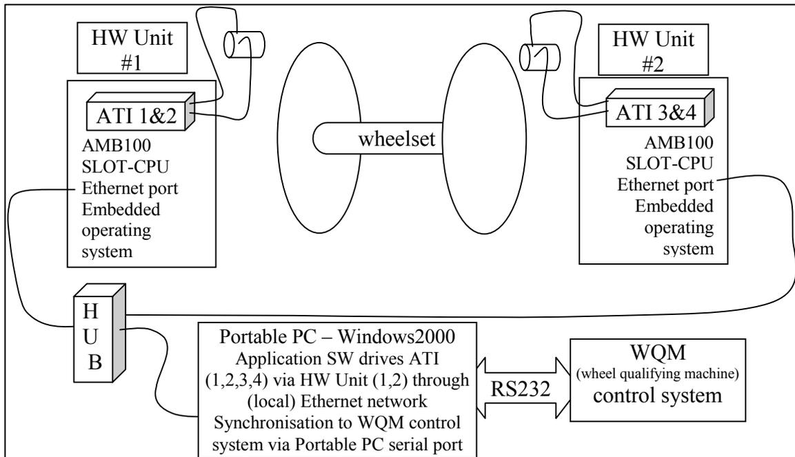
Fig.5 – Architecture of an Ecomat-ST synchronized to the machine allowing wheelset qualification.
