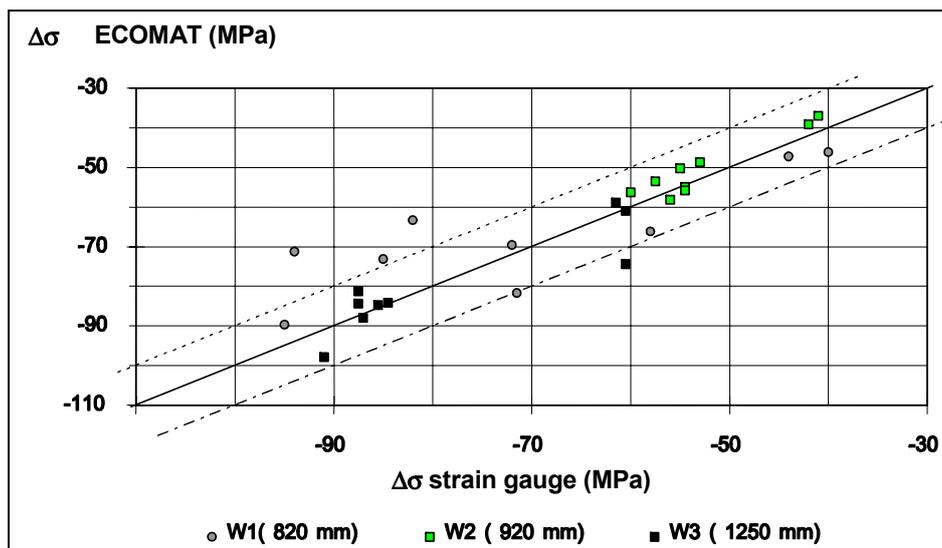
**Fig.1** – Comparison between Ecomat-ST and strain gauge during the sectioning test of new wheels
