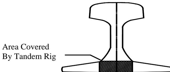
FIG.4- Area Covered by Scan Single 45° Probe for Rail Lower Web and Foot
