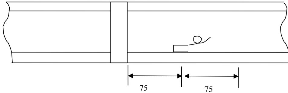
FIG.9- Single 70° Probe Location for Rail Ankle Scanning
