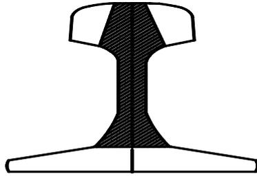
FIG.1- Area covered by Tandem Probe Scan for Rail Head and Web
