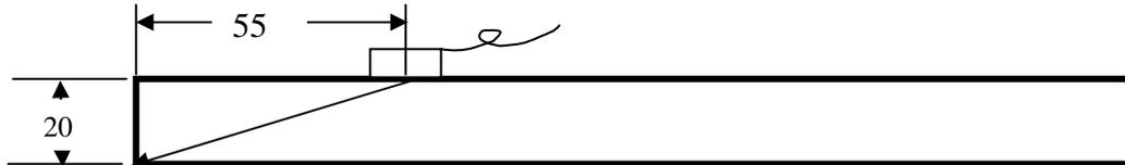
FIG.7- Single 70° Probe Setting Test Sensitivity for Rail Foot Scanning
