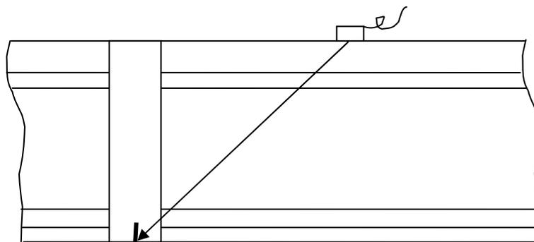
FIG.5- Single 45° Probe for Lower Web and Foot Scanning
