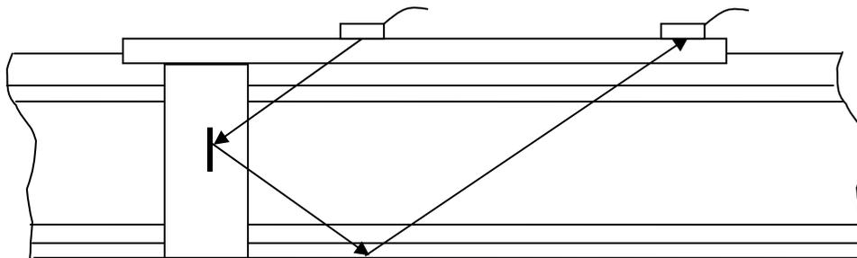
FIG.3- Tandem Probe Rig Scan Arrangement for Vertical Defect Scanning
