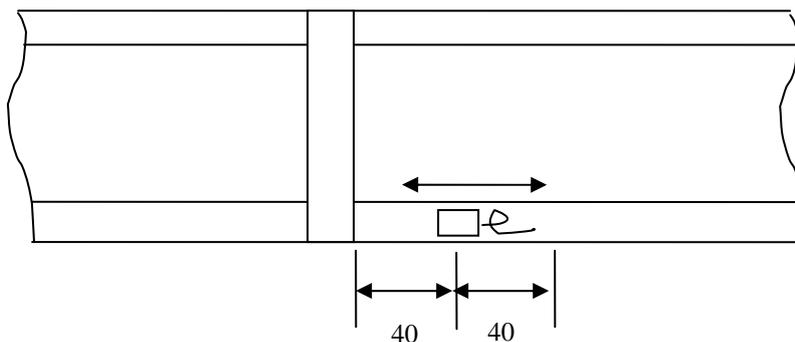
FIG.8- Single 70° Probe Movement for Rail Foot Toe Scanning
