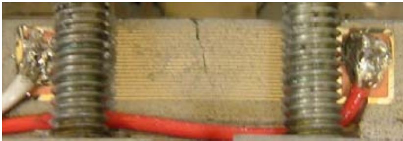
Figure 3: Crack Propagation Gage
