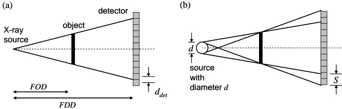
**Figure 4:** Geometric magnification of a CT setup, for an explanation of the symbols see text.
