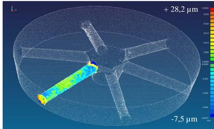
**Figure 7:** Reconstruction of the six injection channels of a fuel injector. The colors in the lower left channel show the deviation from a conical profile.
