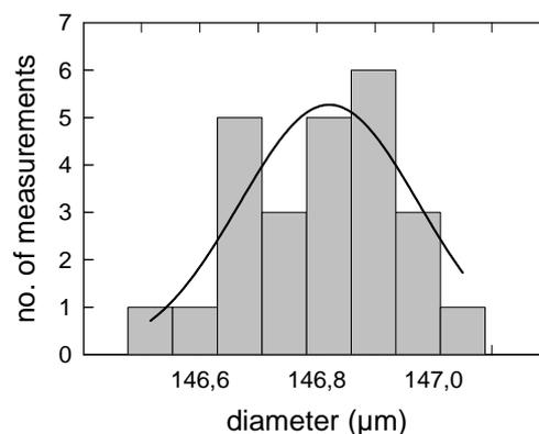
**Figure 8:** Histogram of 25 measurements of the diameter of an injection channel.
