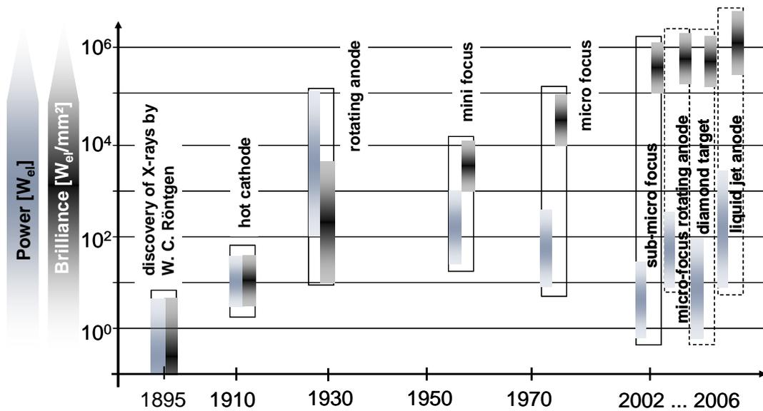
**Figure 5:** Development of X-ray tube performance: Following the discovery of X-rays in 1895, the brilliance developed by about six orders of magnitude due to the design of new X-ray sources. Latest developments represented within a dashed box are not yet commercially available. For reasons of comparability of literature data, the brilliance is here, in contrast to Eq.(1), based on the electrical power  $P_{el}$  per target area.
