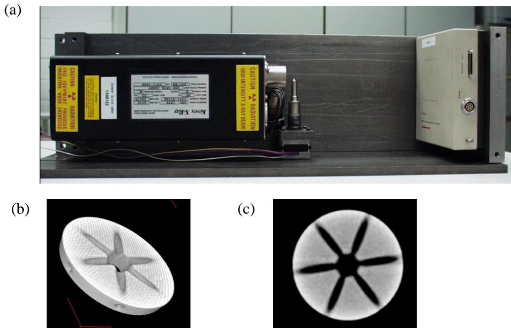
**Figure 9:** a) Mini-CT System with part of the housing removed for visibility of the components. Left: X-ray source, center: manipulator with sample (fuel injector), right: detector. Footprint  $55 \times 18 \text{ cm}^2$ , b) 3D picture and c) projection of a slice of an injector obtained from CT. Diameter of the cross section is approx. 2 mm.
