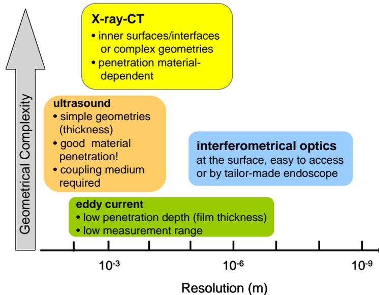
**Figure 2:** Classification of the non-destructive, geometrical measurement techniques discussed in fig. 1. according to geometrical complexity and resolution.
