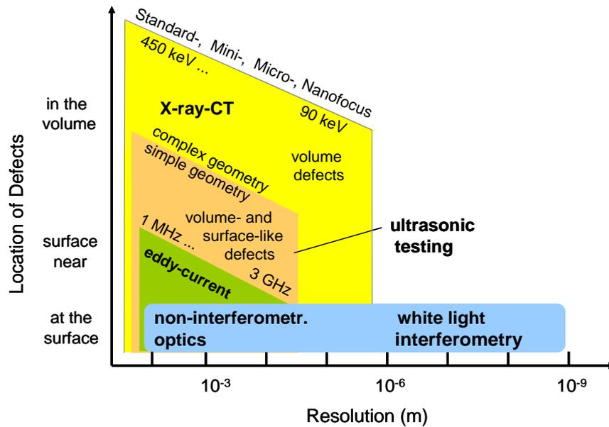
**Figure 1:** Classification and comparison of X-ray CT, ultrasonic testing, eddy current and optical measurement techniques (denoted as non-interferometrical optics and white light interferometry) according to detectable defect location and spatial resolution.
