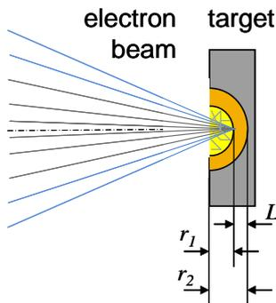
**Figure 6:** Simplified model of heat dissipation in a target.
