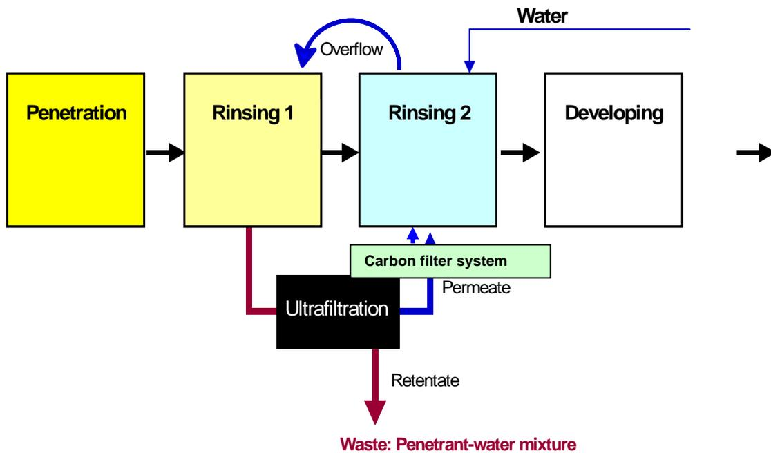
Figure 2: Flow chart of a penetration process with ultra filtration
