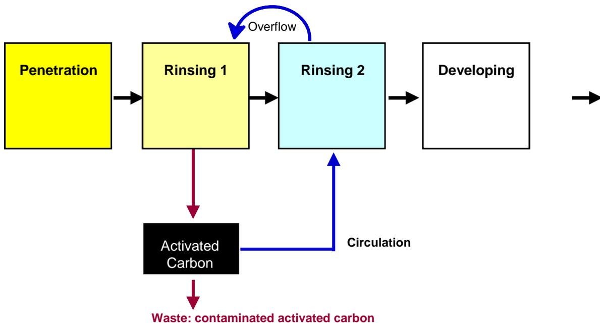
**Figure 1:** Flow chart of a penetration process with activated carbon absorber.
