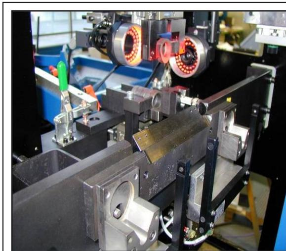
**Fig. 10a:** Vision system in the cam testing station
