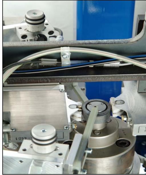
**Fig. 11b:** Eddy current crack test in four zones
