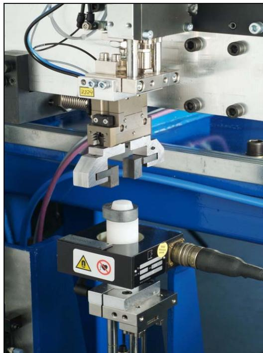
**Fig. 12b:** Hardness testing of a cam with FOERSTER MAGNATEST D
