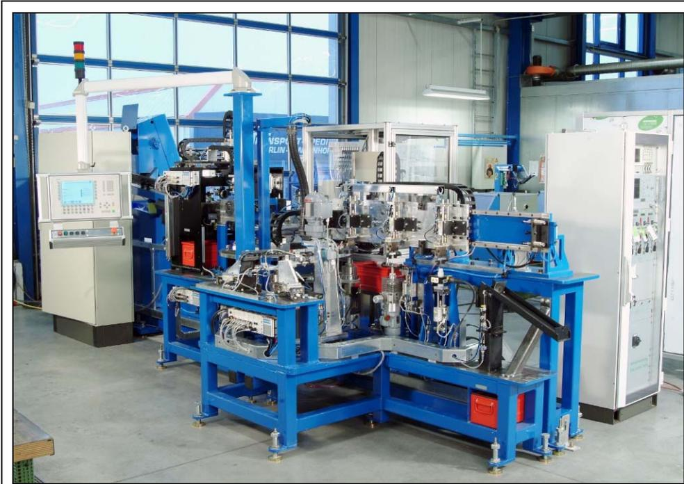
**Fig. 9:** FOERSTER single cam testing station
