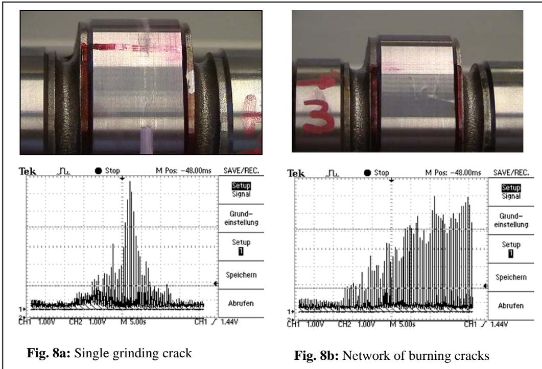
**Fig. 8a:** Single grinding crack
