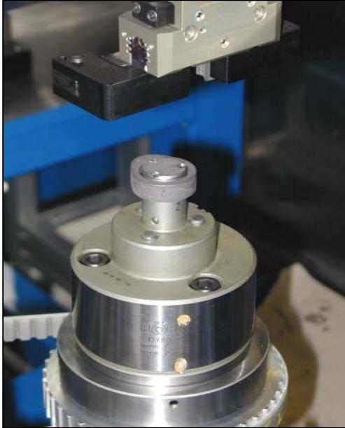
**Fig. 11a:** Cam on the clamping mandrel
