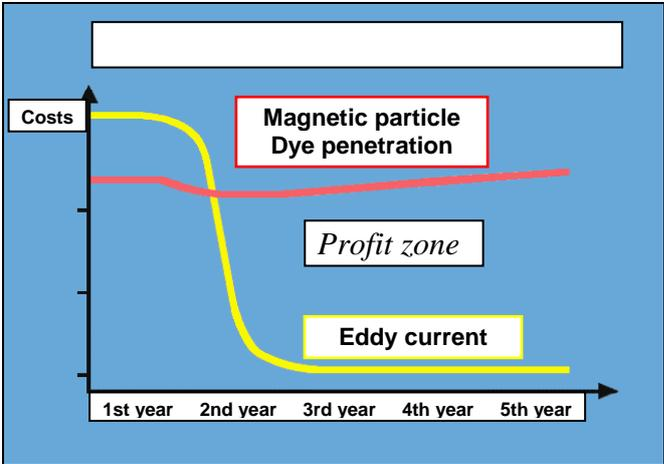
**Fig. 1:** Cost comparison for the use of the eddy current method in relation to the magnetic particle inspection and dye penetration methods.
