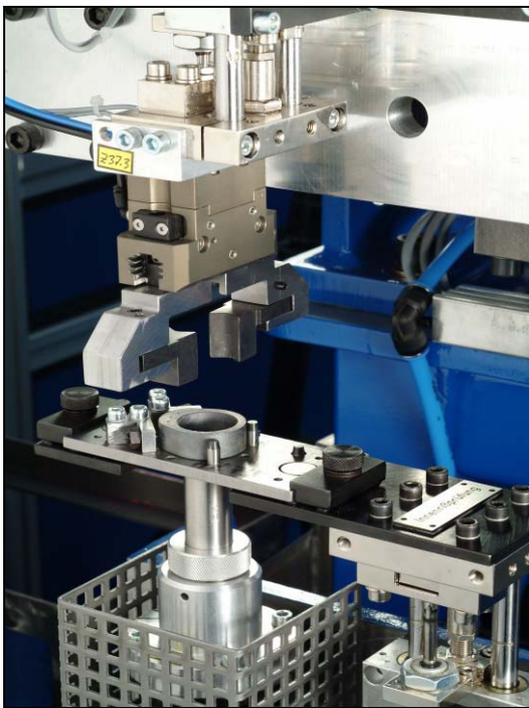
**Fig. 12a:** Eddy current testing within the cam bore hole
