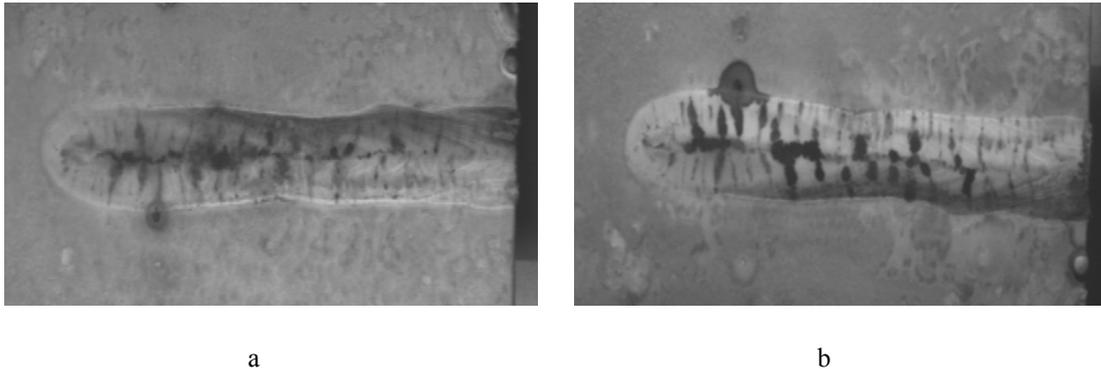
Fig. 1. Growth of a defect indication in welded seam at increase of penetrant "Pion" dwell time: a - 1 min, b - 10 min.
