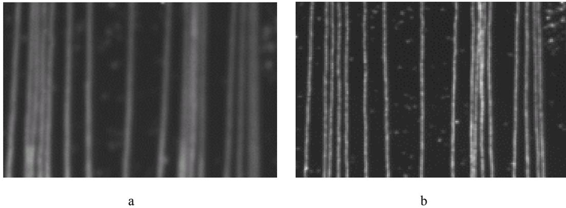
Fig. 4. Development of the cracks without heating (a) and using warm airflow (b).
