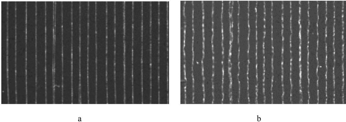
Fig. 2. Dynamic effect at the close distance between spray nozzle and test surface.
