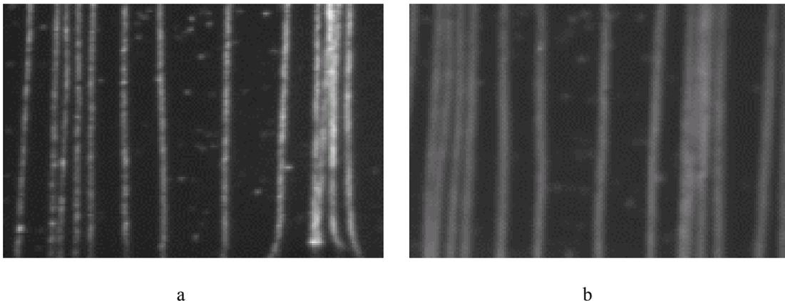
Fig. 3. Defect's indications in test panel: developers with high (a) and low (b) developer layer drying speed.
