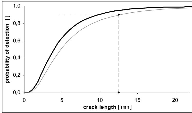
**Figure 3.** Estimation of reliably detectable crack length
