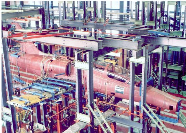
**Figure 1.** Full-scale fatigue test
