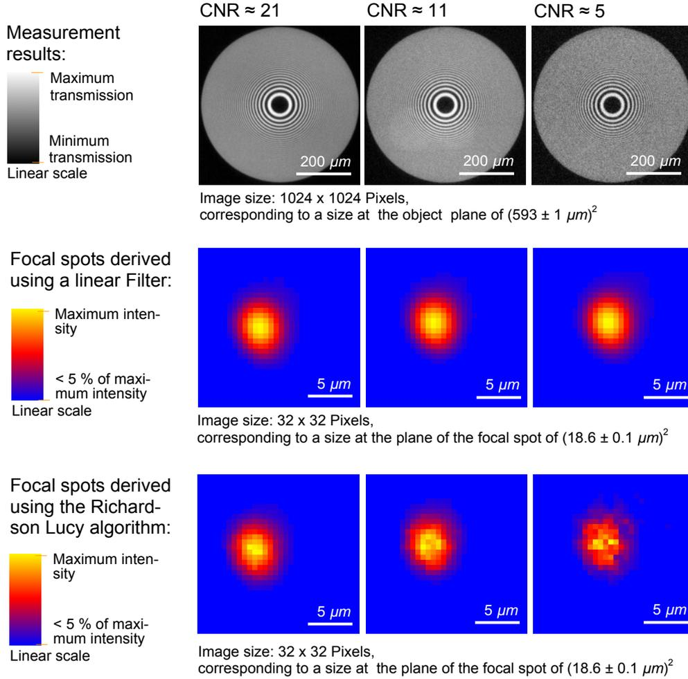
FIG. 5: Results of transmission measurements of the ring test pattern for three independent measurements with different total exposure times yielding contrast to noise ratios of 21, 11 and 5, focal spots derived using a linear filter according to Eq. (3) and Eq. (5) which is similar to the Wiener filter and focal spots derived using the Richardson Lucy algorithm with 500 iterations. The X-ray tube was operated at 50 kV and 60  $\mu\text{A}$ .
