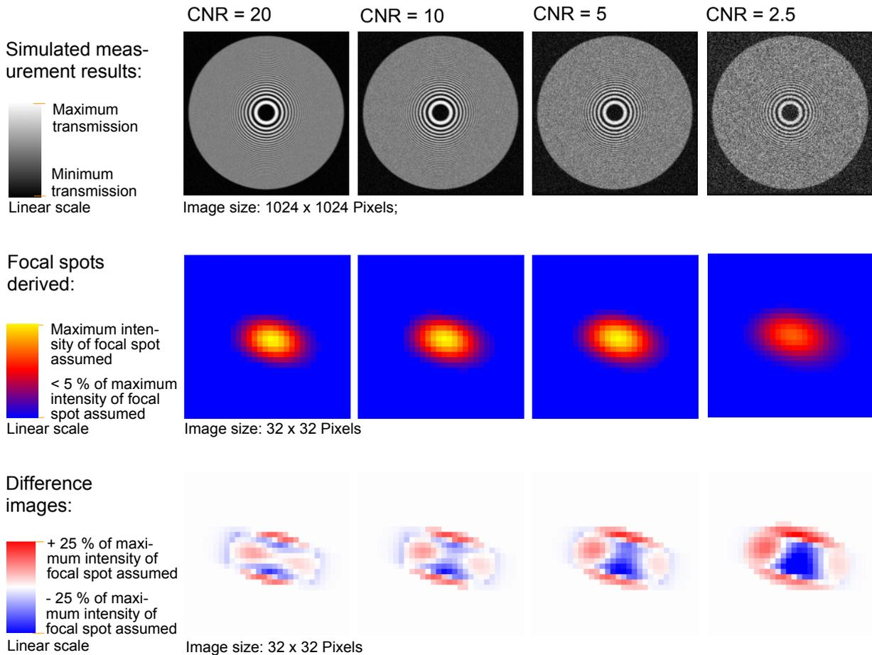
FIG. 3: Results of simulated transmission measurements of the ring pattern with a CNR of 20, 10, 5 and 2.5, focal spots derived from these simulated measurements using the Wiener filter according to Eq. (3) and Eq. (4) and difference images showing the deviation from the focal spot assumed.
