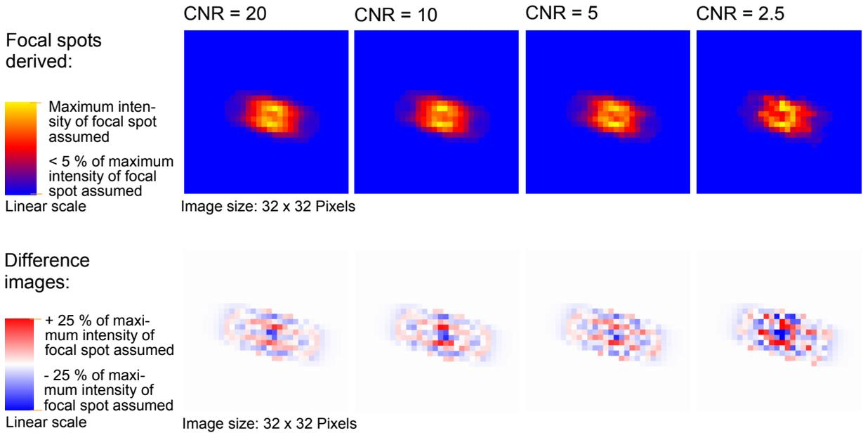
FIG. 4: Focal spots derived from simulated transmission measurements of the ring pattern with a CNR of 20, 10, 5 and 2.5 using the Richardson Lucy algorithm and difference images showing the deviation from the focal spot assumed.
