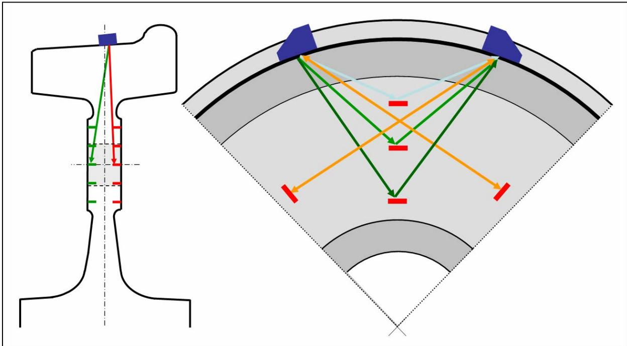
**Figure 4** Example 2 - Testing of Discs Using Matrix Array Probes
