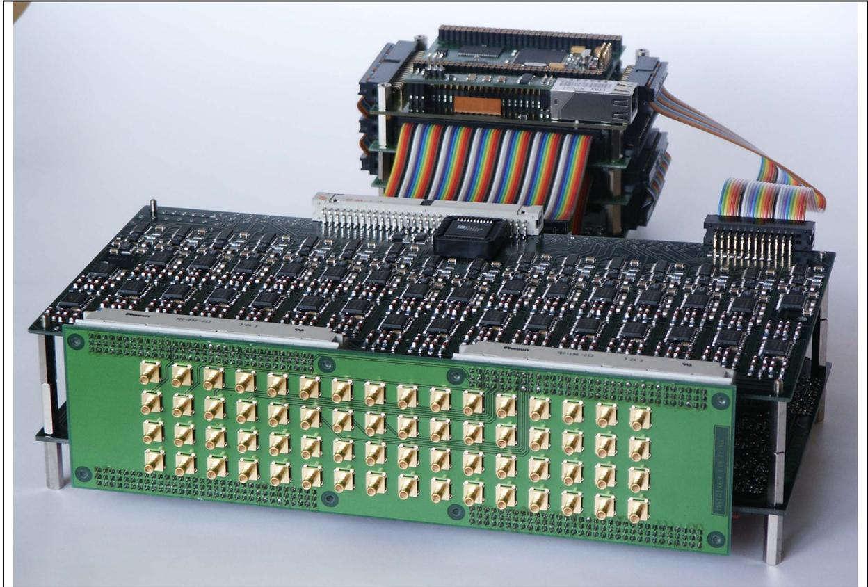
**Figure 2** Ultrasonic Subassembly of MATRIX64 Testing System
