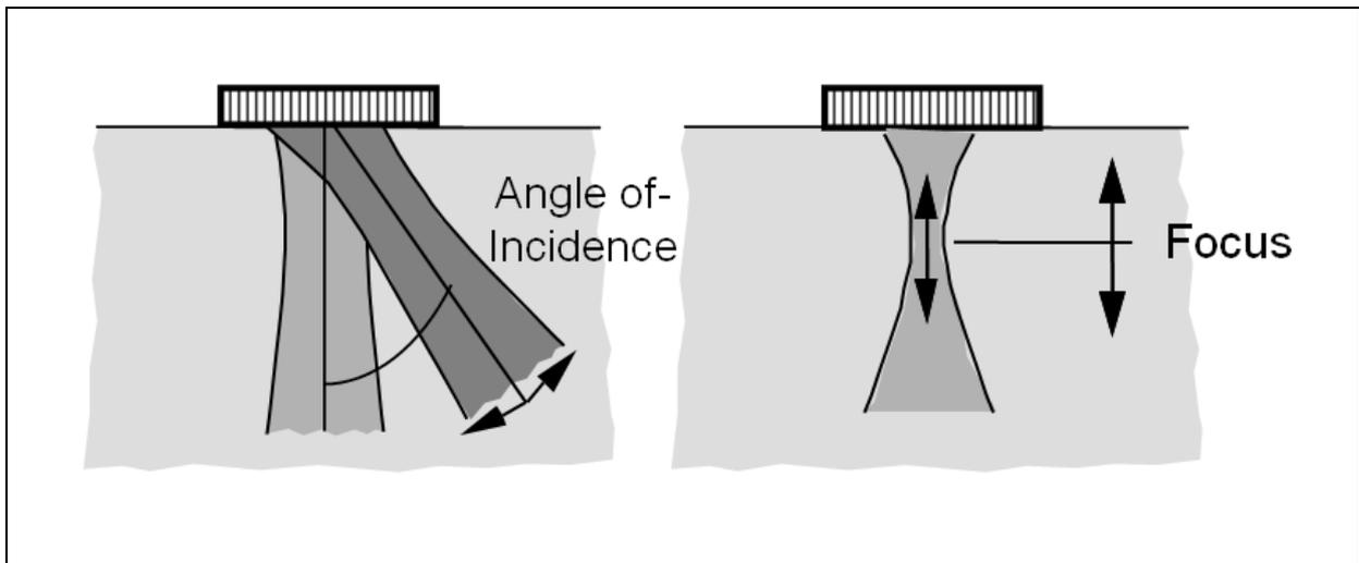
**Figure 1** Phased Array Principle
