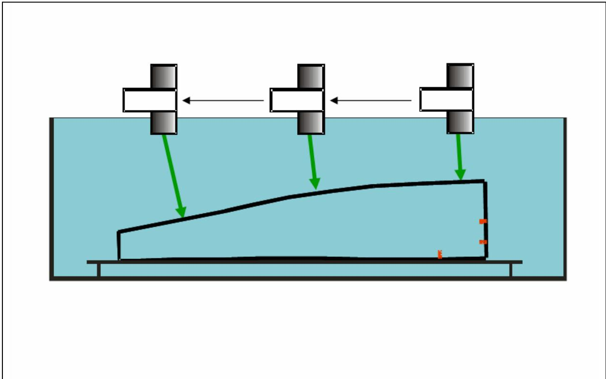
**Figure 3** Exampe 1 - Immersion Technique Using Matrix Array Probe
