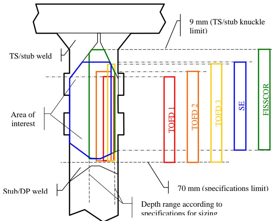
Figure 9 – Wall section inspection capability by transducer
