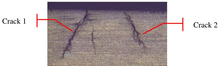
Figure 8 – Tilted SCC on one side of AREVA NP’s mock-up
