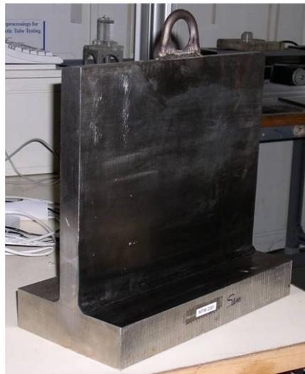
Figure 2 – Welded stub/DP mock-up
