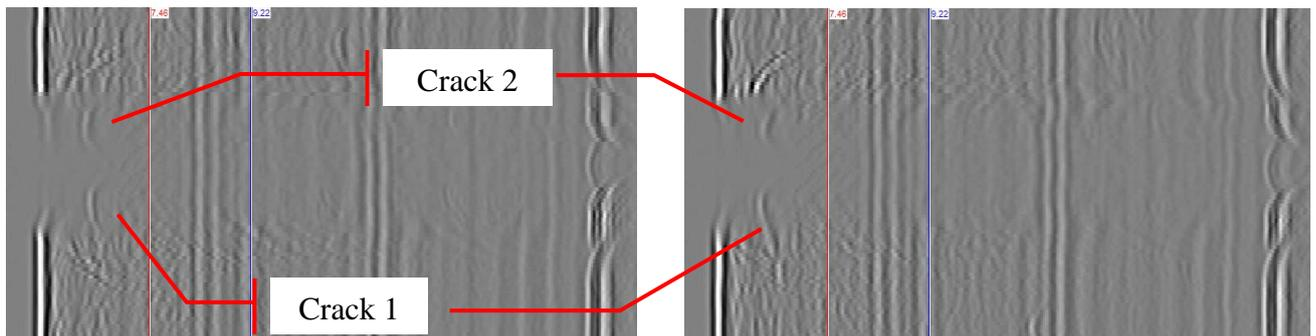
Figure 7 – TOFD PCS 14 mm – SCC mock-up
