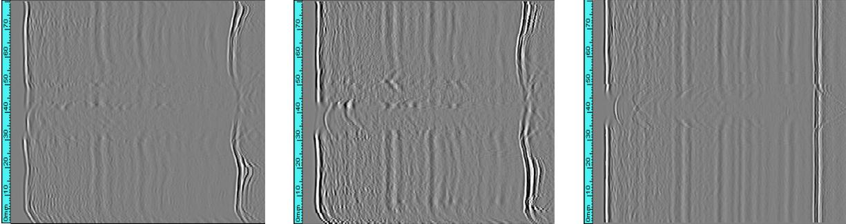
Figure 6 a) : EDM 2 mm in a weld    b) : EDM 4 mm in a weld    c) : EDM 4 mm in base metal
