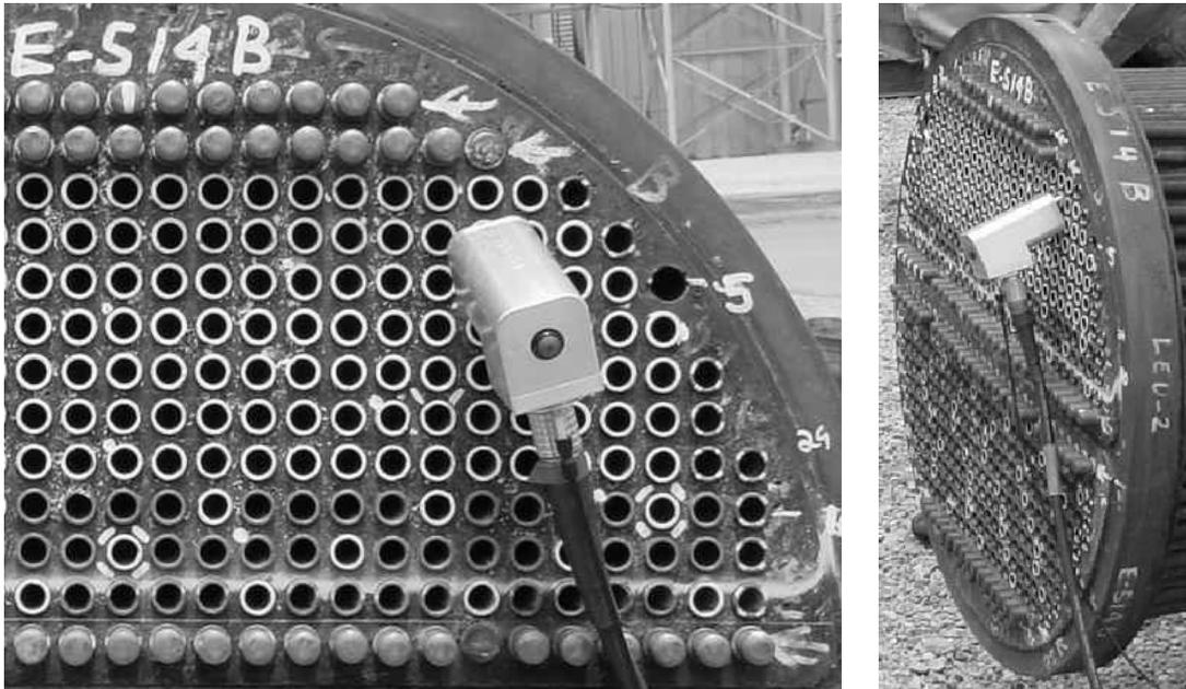
**Figure 2.** Tube screening system with probe-head inserted the tube, only handle is visible.
