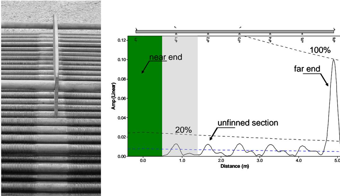
**Figure 9.** Integral fin tubing (left) and example result (right).
