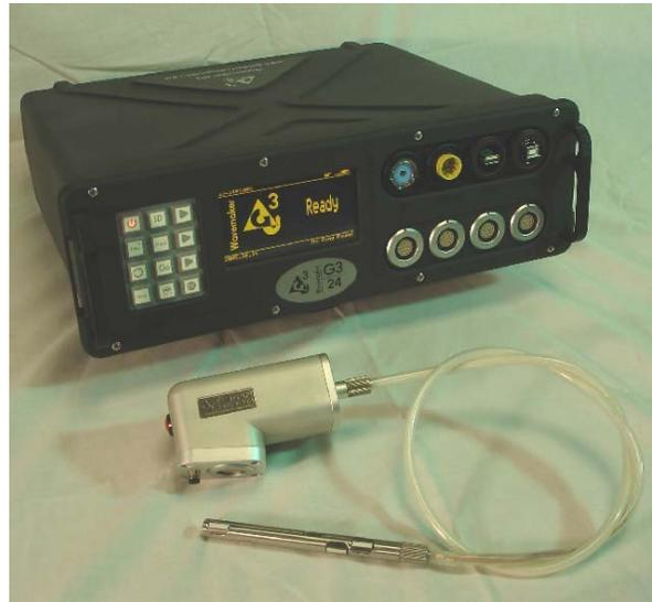
**Figure 1.** Wavemaker G3 and 3/4 inch probe-head.
