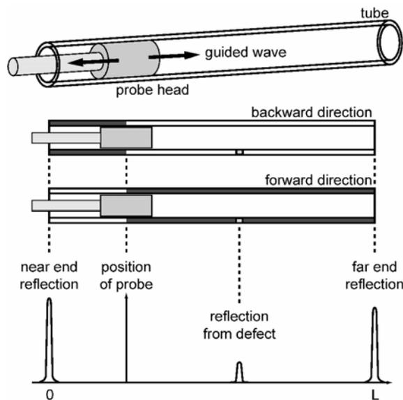
**Figure 3.** Schematic of the principle of test in a tube with defect.
