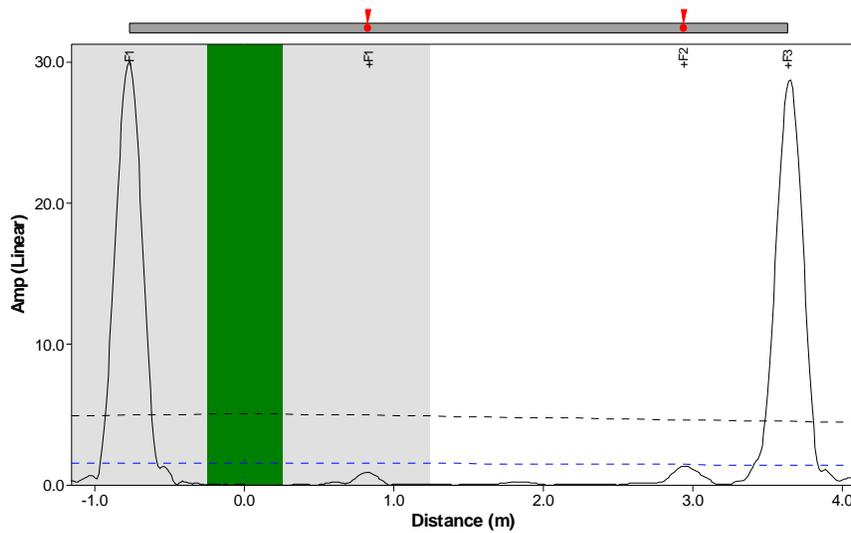
**Figure 6.** Example result from a tube with two defects (+F1 approximately 8%, +F2 approximately 10% cross-section loss).
