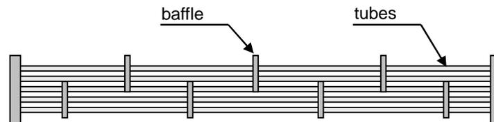
**Figure 7.** Schematic of a heat exchanger (side view).
