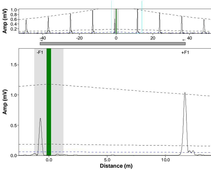
**Figure 5.** Example result from a tube with no defect.
