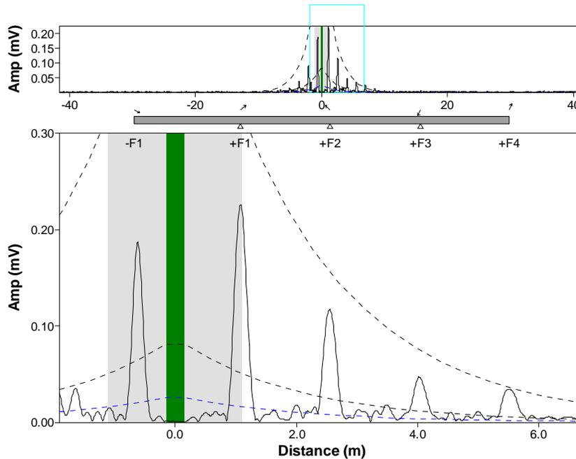
**Figure 8.** Heat exchanger tube with tight baffle plates.
