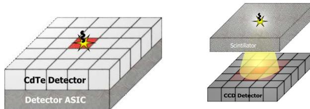
Direct-direct CdTe detector (left) and an indirect-direct CCDs or TFTs (right)
