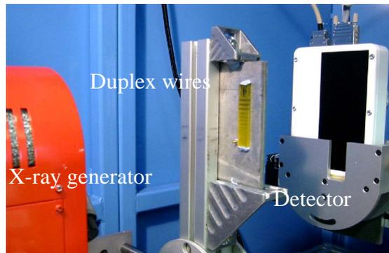
The duplex wire is one of the standard radiographic techniques used to measure unsharpness. Unfortunately, for this experiment, the smallest wires were always resolved, due to the small focal spot size of the generator.
