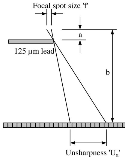
The focal spot size is measured by placing a 125µm lead sheet, with a sharp edge, close to the focal spot, to produce a large amount of unsharpness. The image is captured and the value of  $U_g$  obtained for that Source to Object Distance 'a'. The value 'a' is then altered and the value of  $U_g$  measured again. This was done for all three focal spot size. The focal spot size can then be calculated from Equation 2, below:
