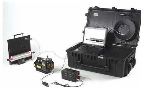
Flat *foX-17* and *foX Rayzor* Portable a-Si Inspection Systems Packaged in a Pelican Case
